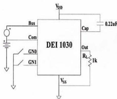
A filter capacitor is used in the RMS-to-DC conversion. A value of at least 0.22  $\mu$ F is recommended. A larger value will reduce the ripple (at 2x the input frequency) at the output.
