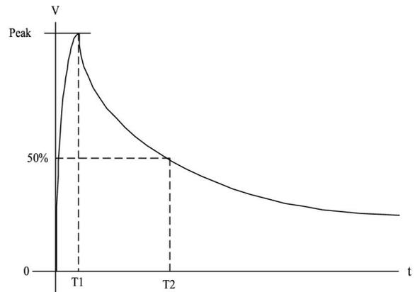
**Figure 6: DO160C/D Voltage Waveform #4**
