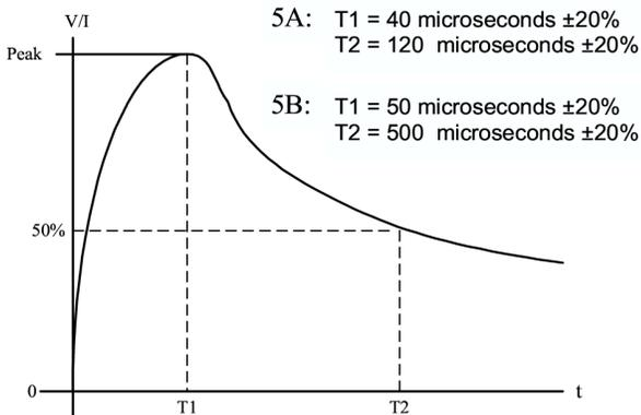
**Figure 7: DO160C/D Voltage Waveform #5**
