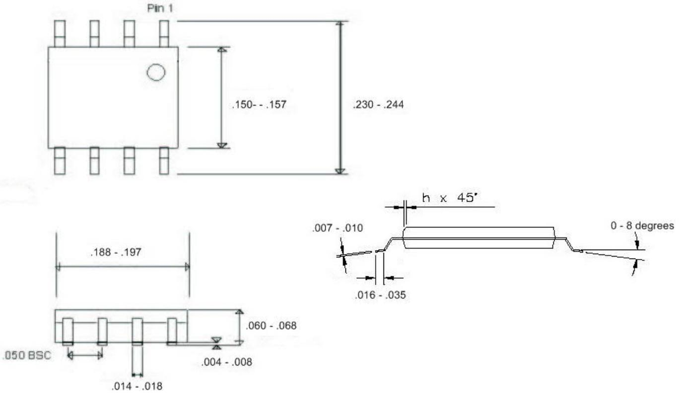
**Figure 8: Mechanical Outline 8 Lead NB SOIC – G Package**
