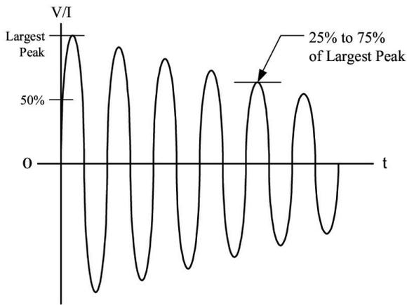
**Figure 5: DO160C/D Voltage Waveform #3**
