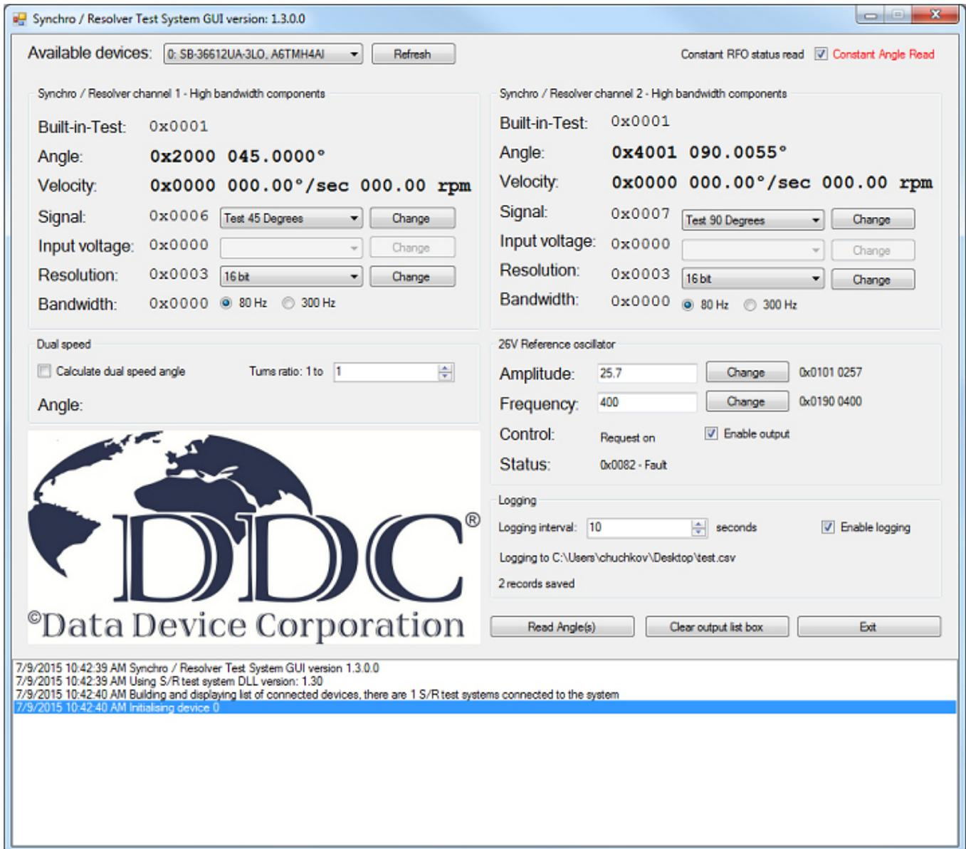
Figure 35. GUI - Data Logging Feature
