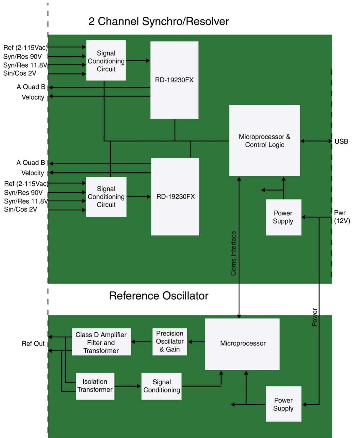
Figure 2. SB-36610UX Block Diagram
