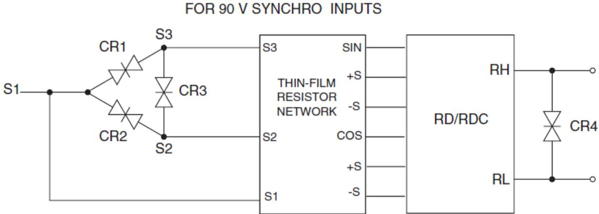
CR1, CR2, CR3, and CR4 are 1.5KE170CA or 1.5KE200C-type bipolar transient voltage suppressors or equivalent.
