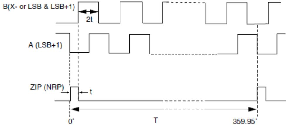
Figure 22. Incremental Encoder Emulation Timing
