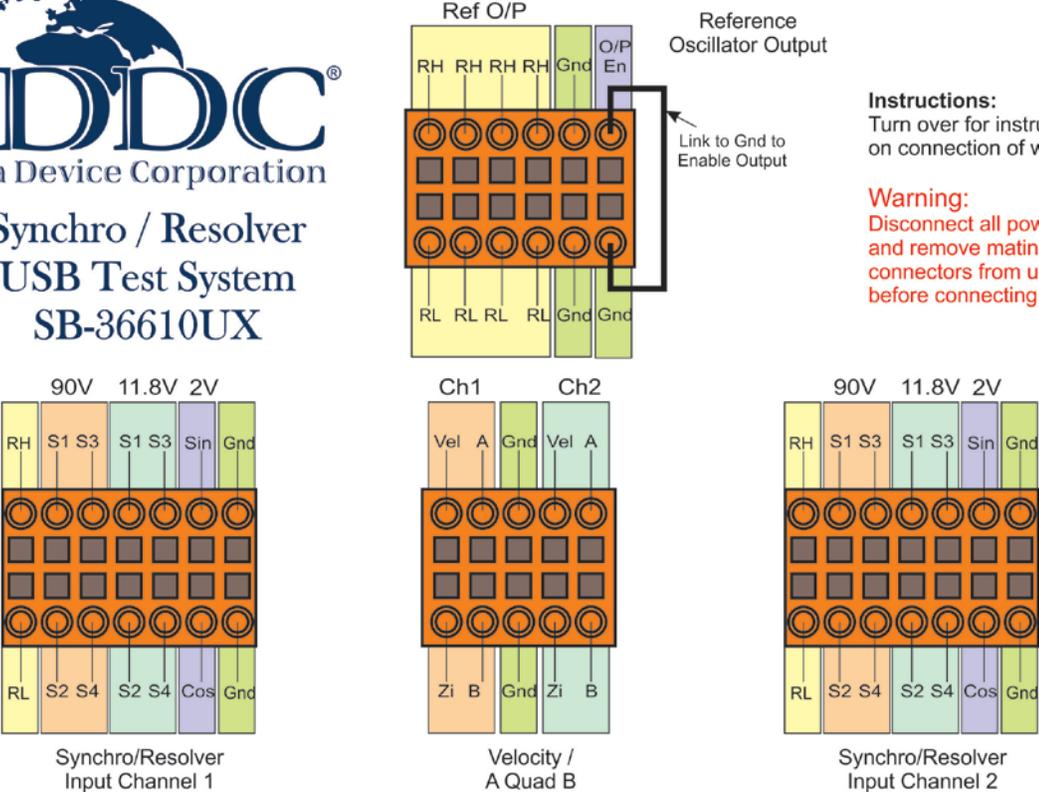
Figure 36. Quick Reference Wiring Guide (Front)
