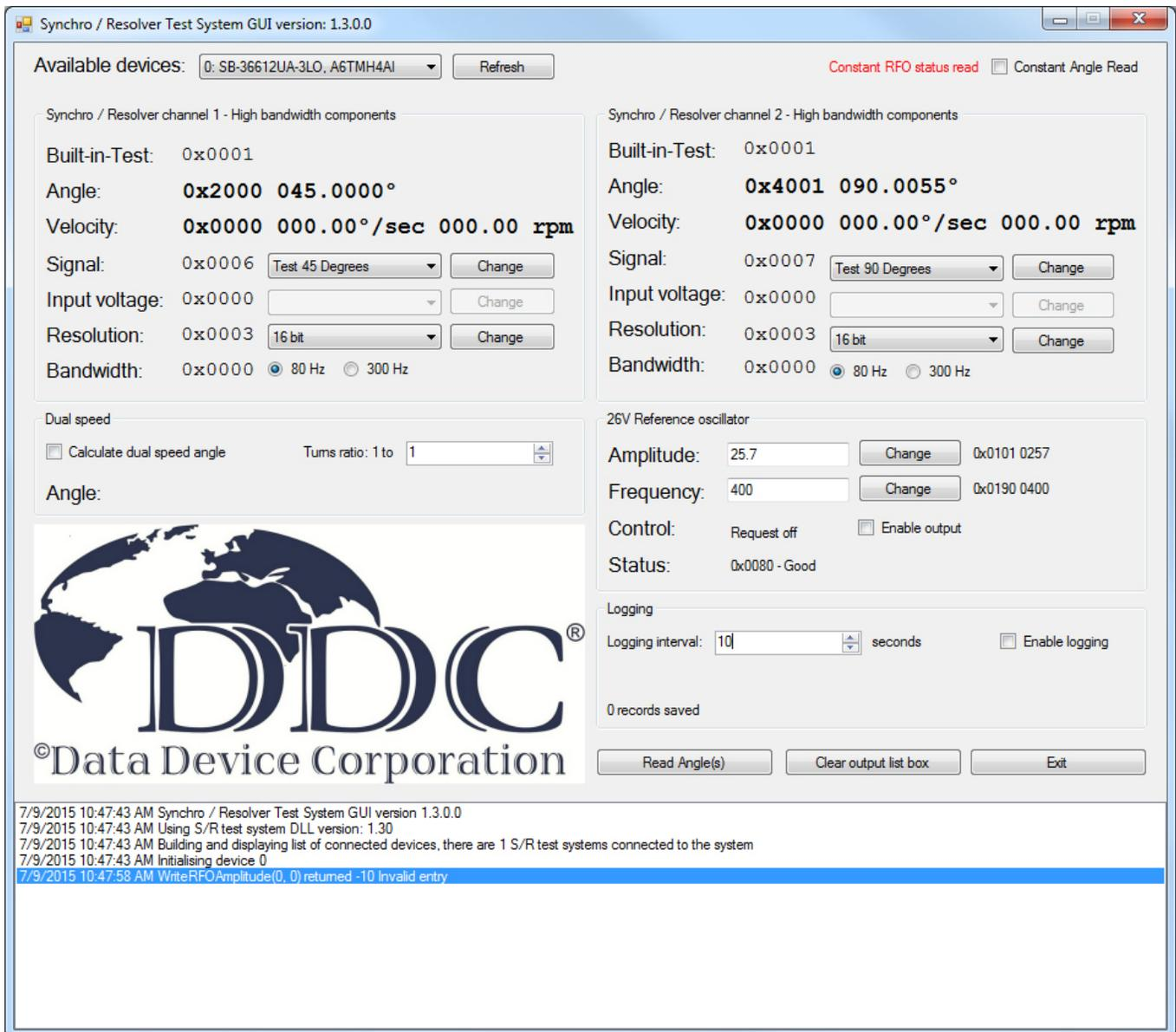
Figure 28. SR Test System GUI
