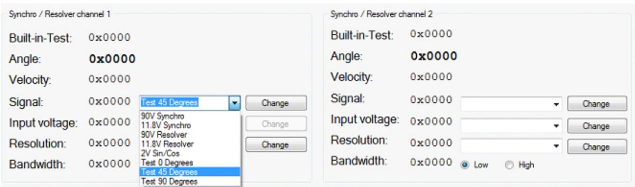
Figure 34. GUI- Self-test Feature
