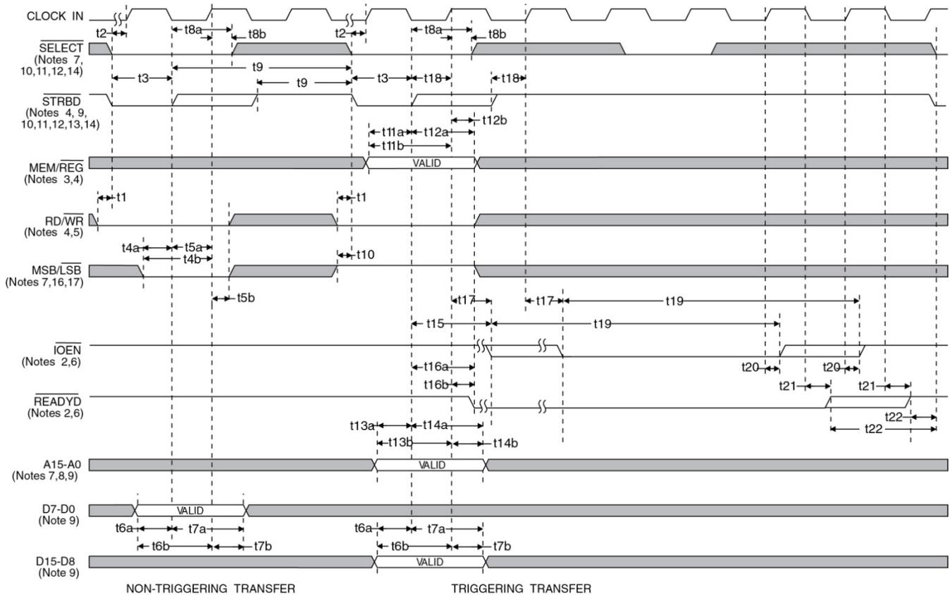
**Figure 31. CPU Writing RAM/Registers (8-Bit, Zero Wait)**
