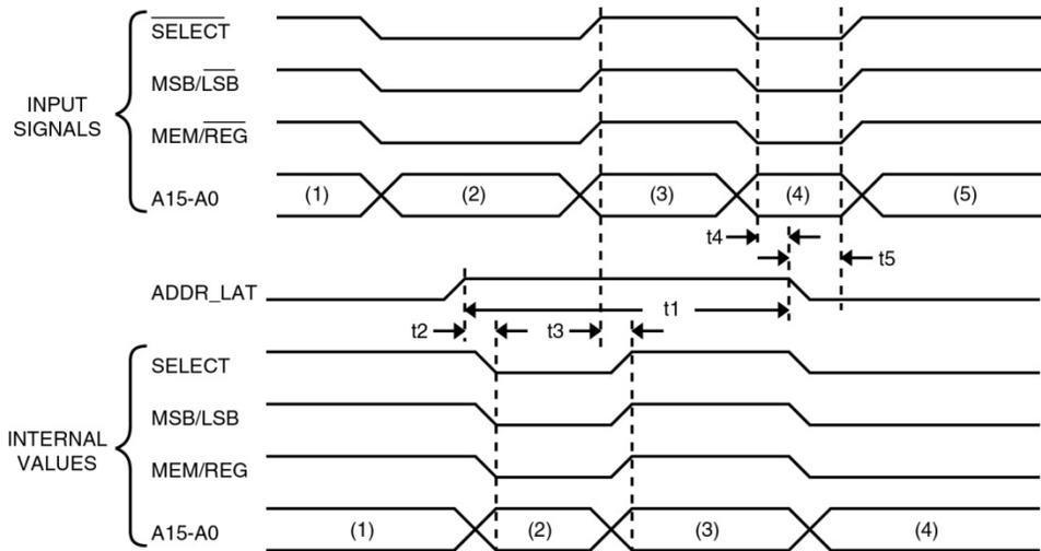
Figure 32. Address Latch Timing
