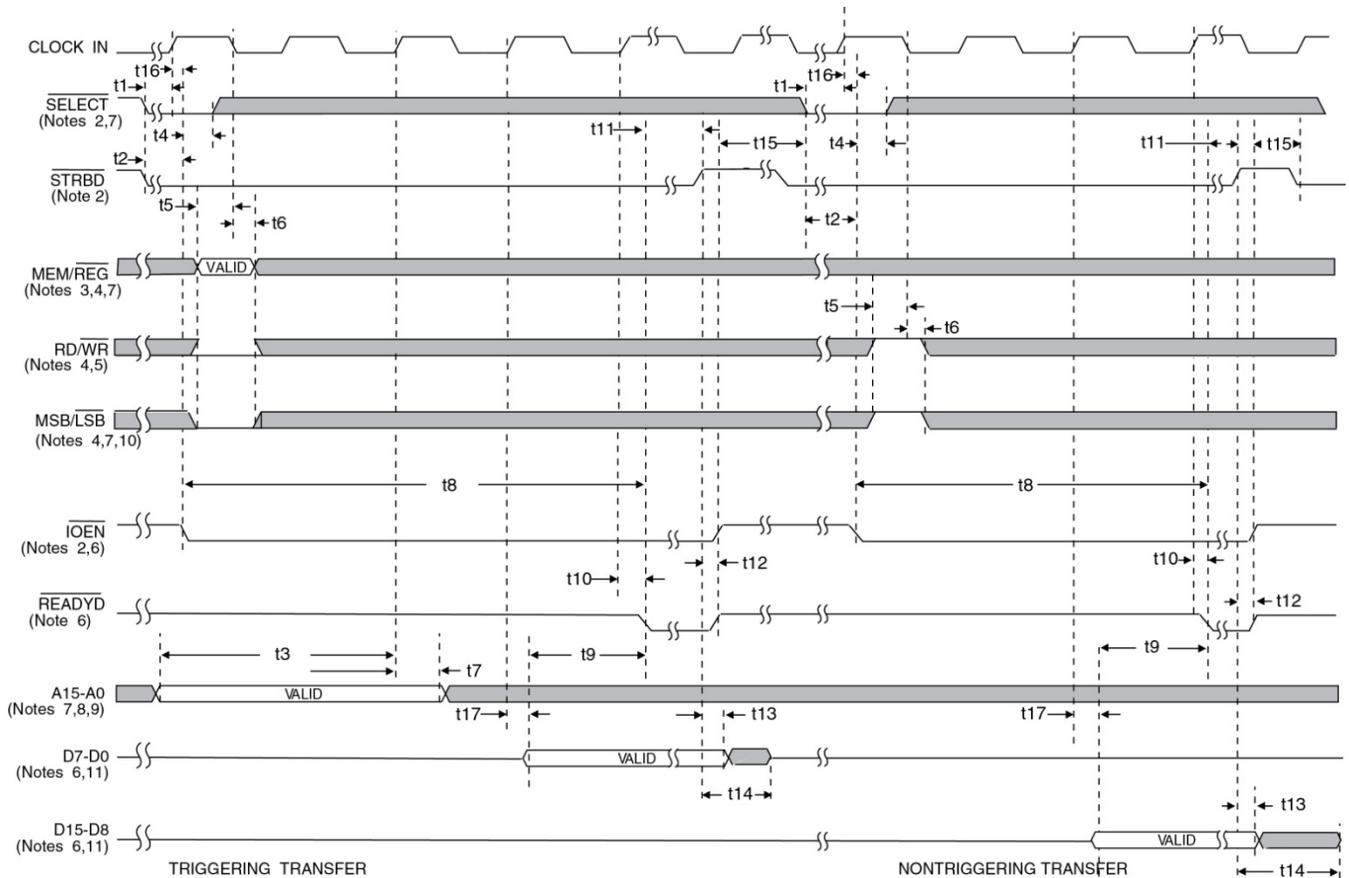
**Figure 28. CPU Reading RAM/Registers (8-Bit, Nonzero Wait)**
