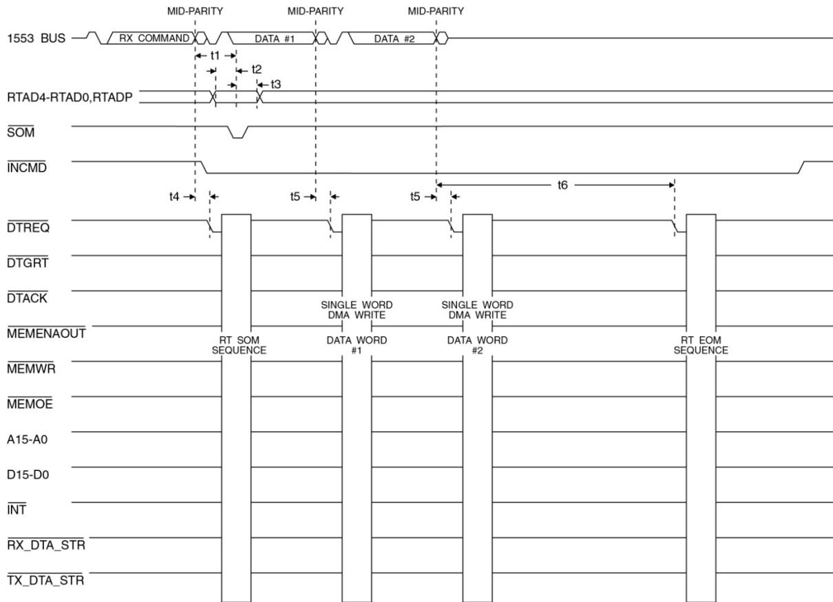
**Figure 58. RT Broadcast Receive Message Timing**
