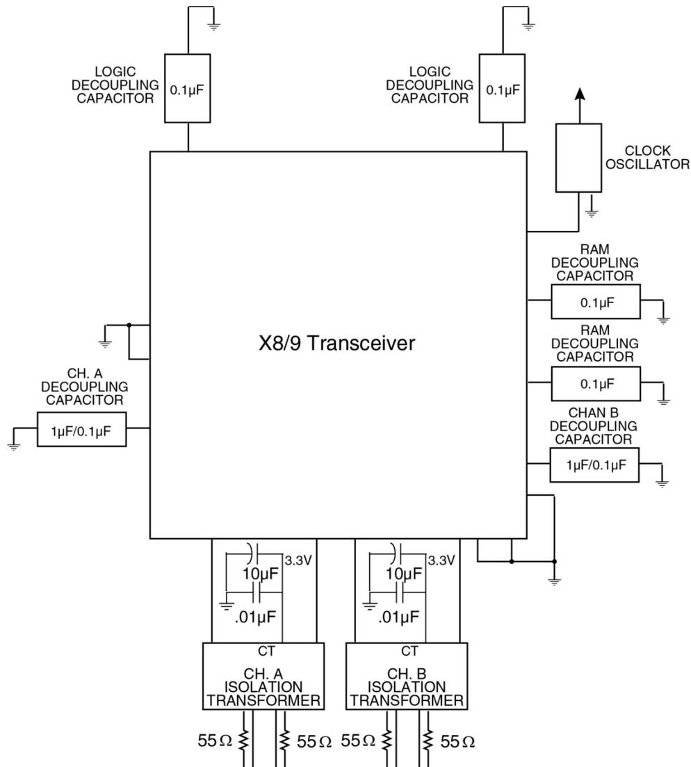
**Figure 11. P.C. Board Layout Example: X8/9 Transceiver**
