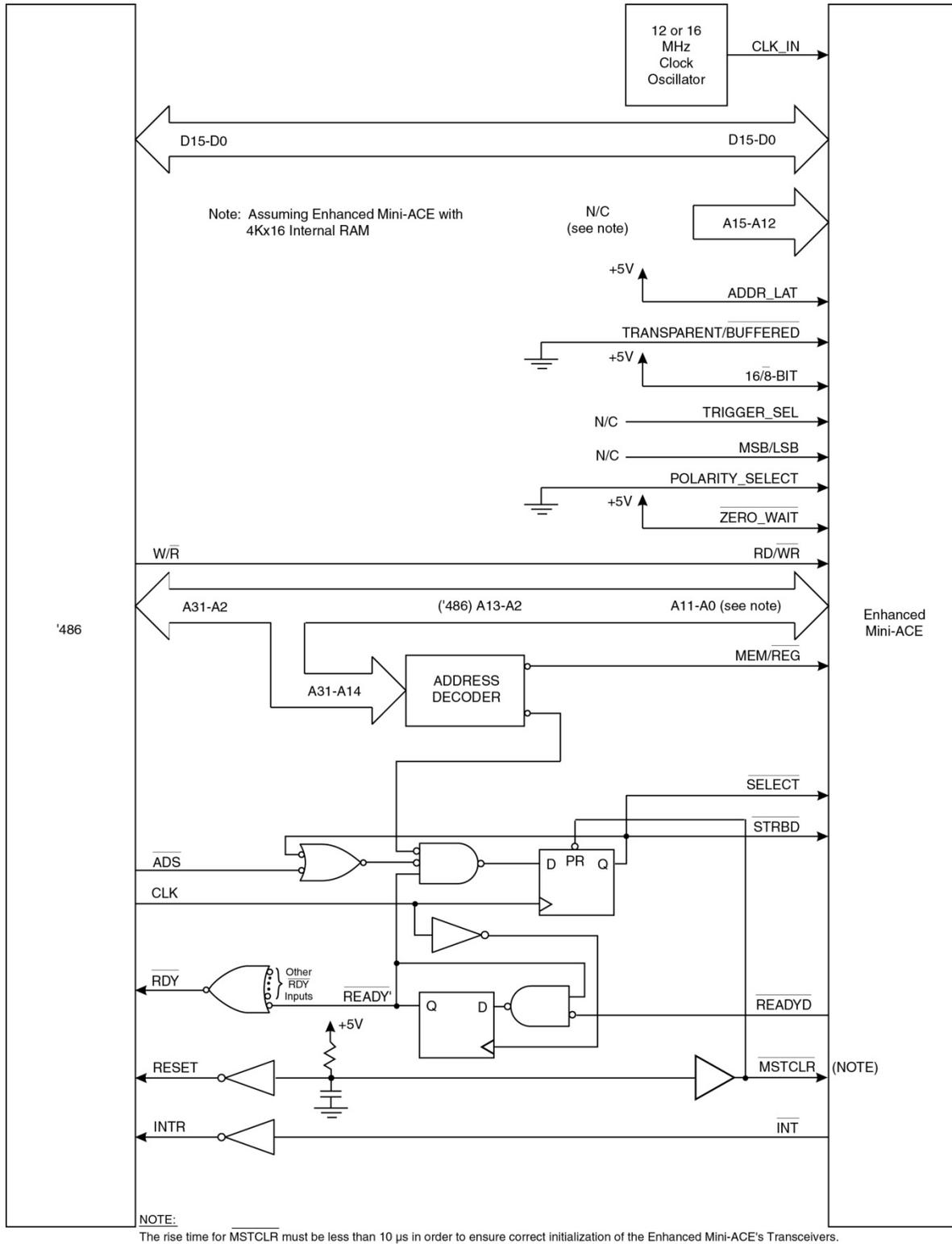
Figure 44. INTEL 80486-to-Enhanced Mini-ACE Interface
