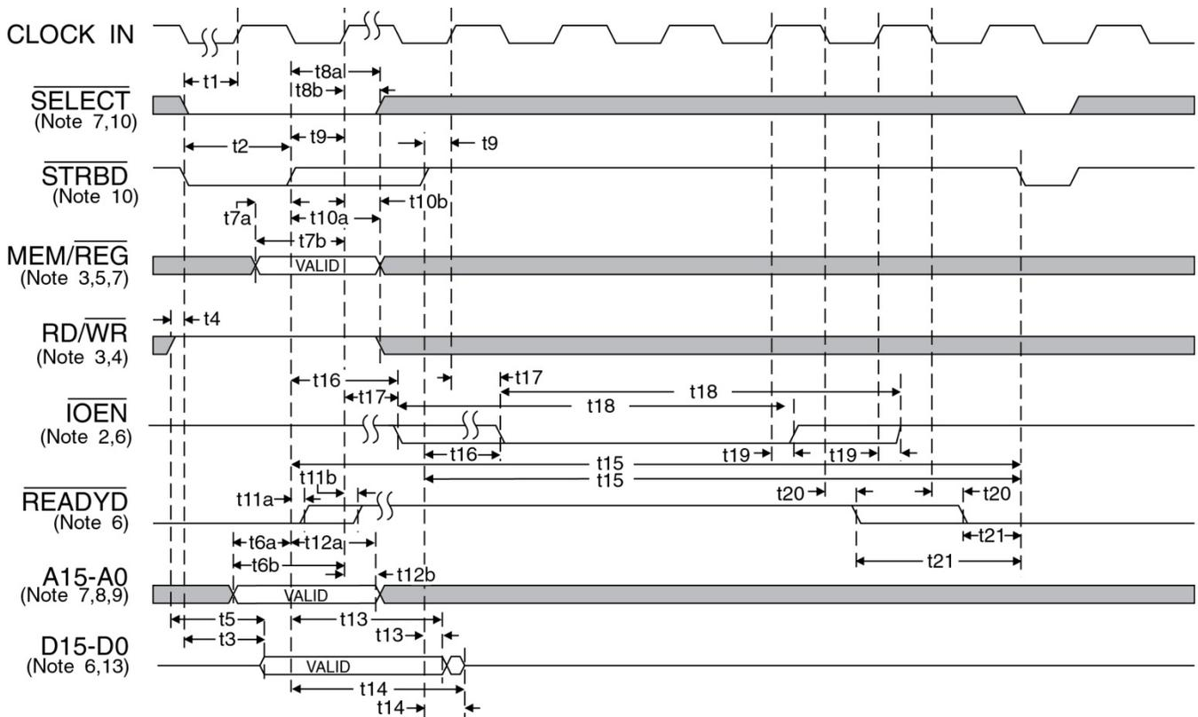
Figure 24. CPU Reading RAM/Registers (16-Bit, Buffered, Zero Wait)
