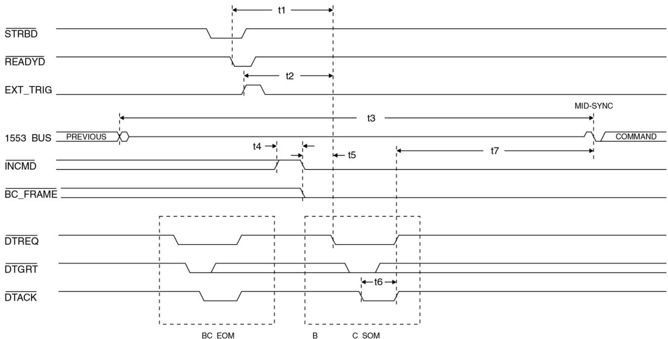
Figure 52. BC Mode Start Timing
