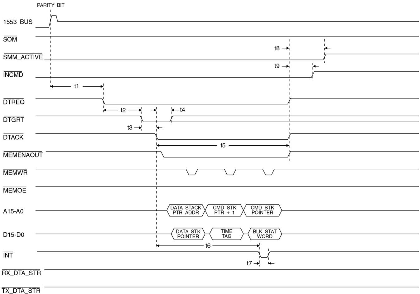
**Figure 66. Message MT End of Message (EOM) Timing**
