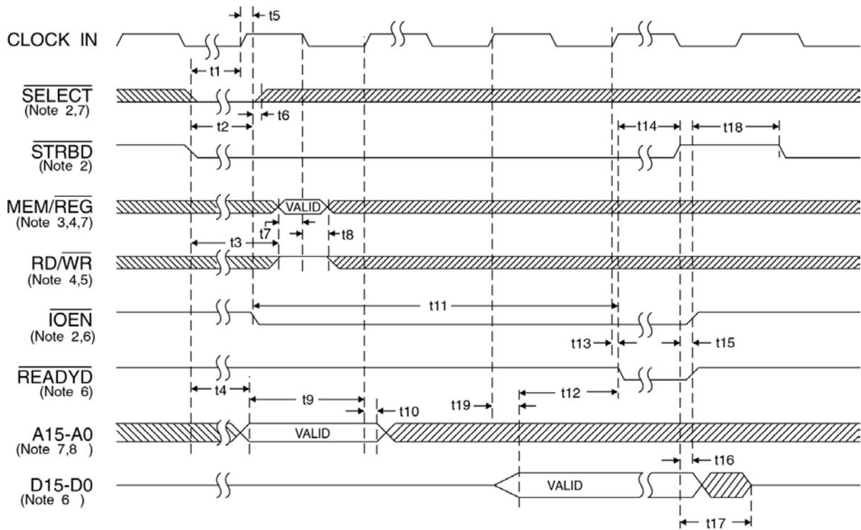
**Figure 22. CPU Reading RAM/Registers (16-Bit, Buffered, Nonzero Wait)**
