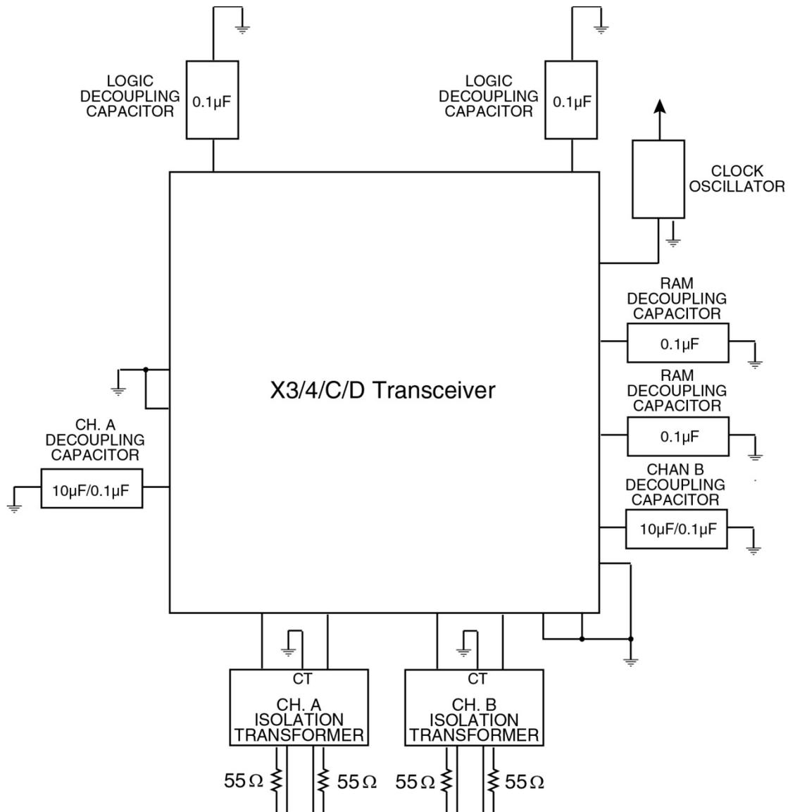
**Figure 10. P.C. Board Layout Example: X3/4/C/D Transceiver**
