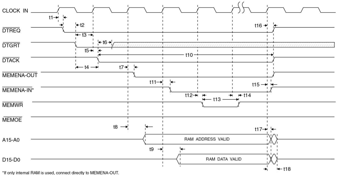
**Figure 47. Enhanced Mini-ACE Single Word DMA Write (Transparent Mode)**
