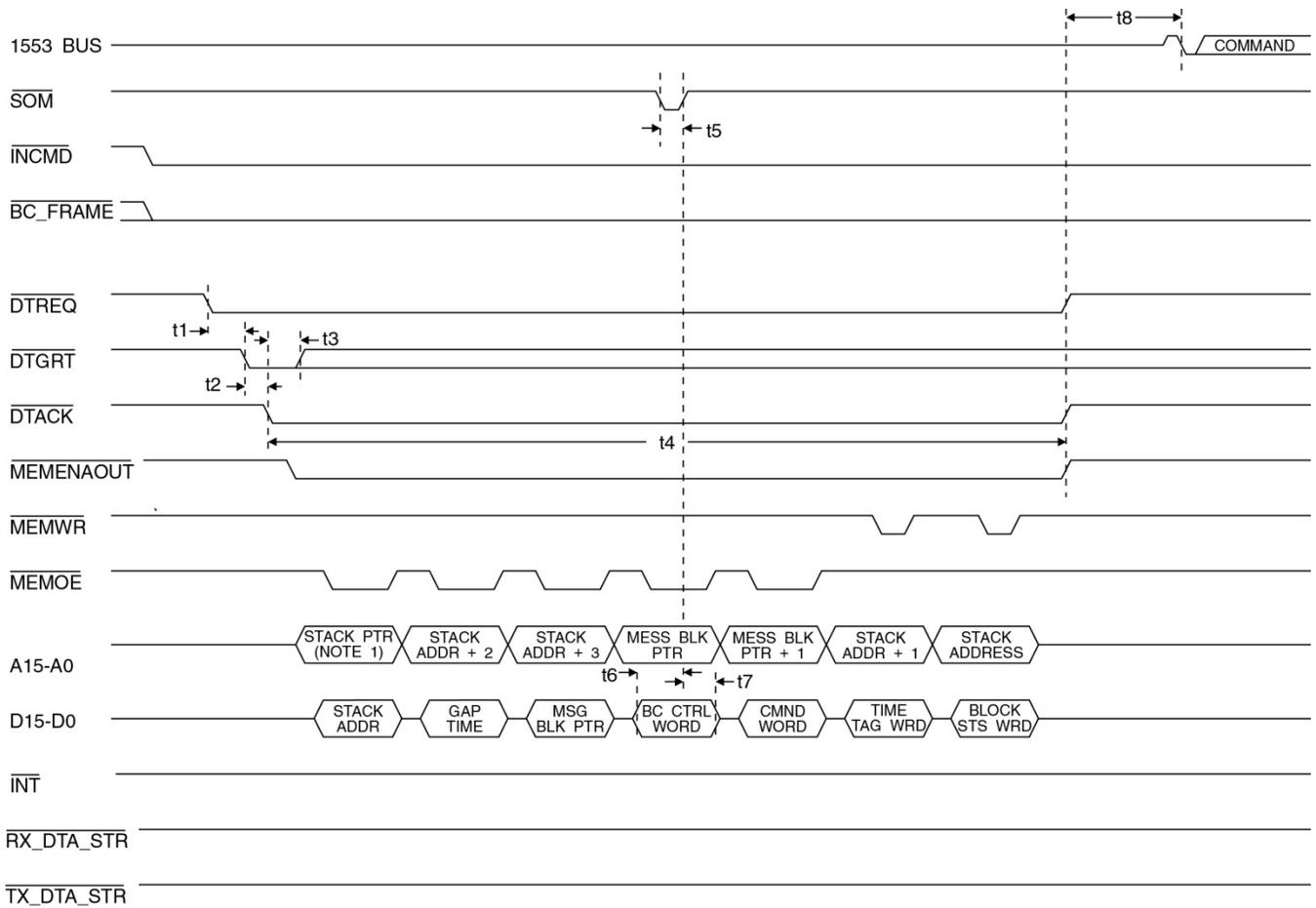
**Figure 53. BC Start of Message (SOM) Sequence Timing**
