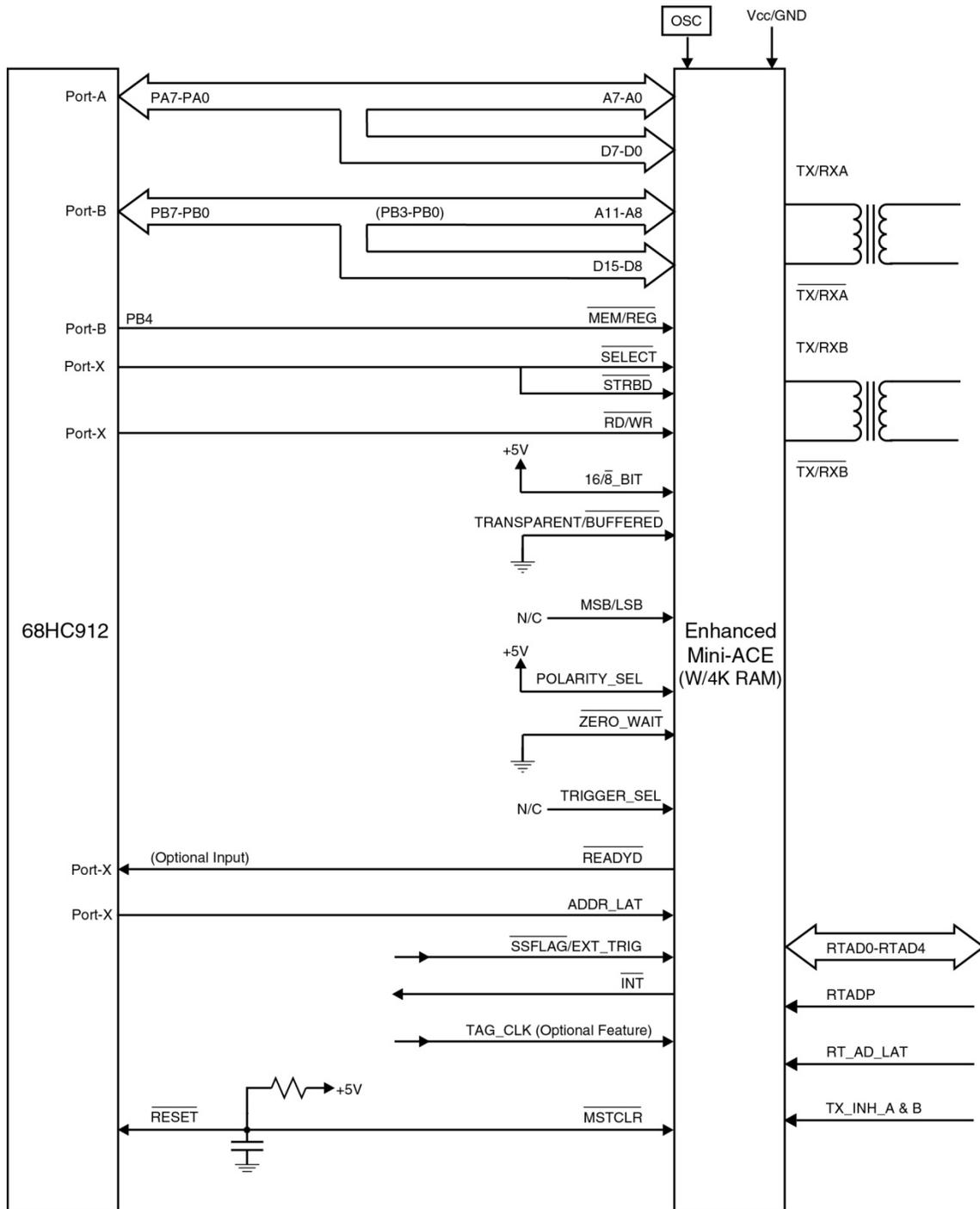
Figure 35. Motorola 68HC912-to-Enhanced Mini-ACE Interface
