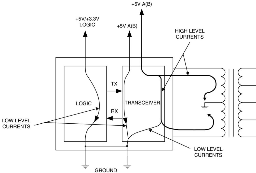
Figure 12. Power/Ground Current Distribution for +5V Transceivers (X3/4 Option)
