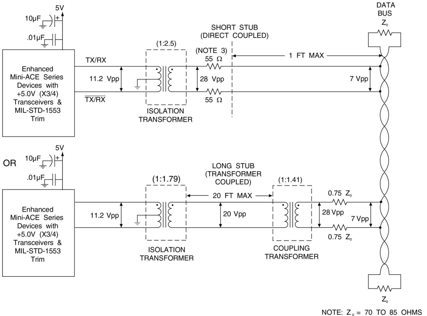
**Figure 4. Enhanced Mini-ACE Series Interface to 1553 Bus (+5.0V Transceivers [X3/4] & MIL-STD-1553 Trim shown)**
