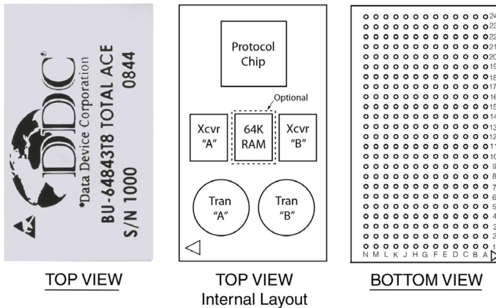
Figure 9. Ball Locations for Total-ACE (BGA Package)
