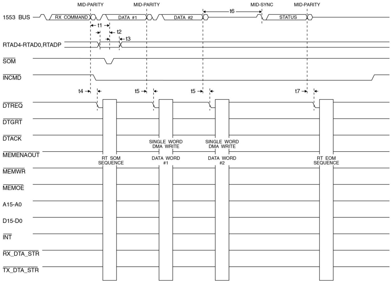
**Figure 56. RT Receive Message Timing**
