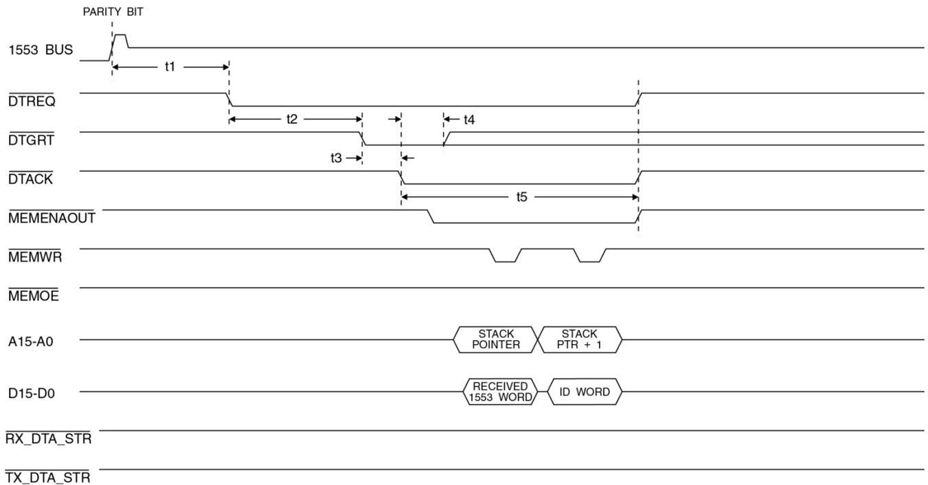
**Figure 68. Word MT Received Word Write Cycle Timing**
