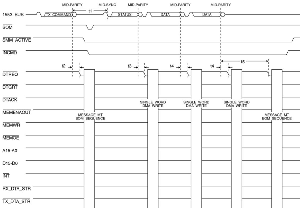
Figure 62. Message MT Transmit Message Timing
