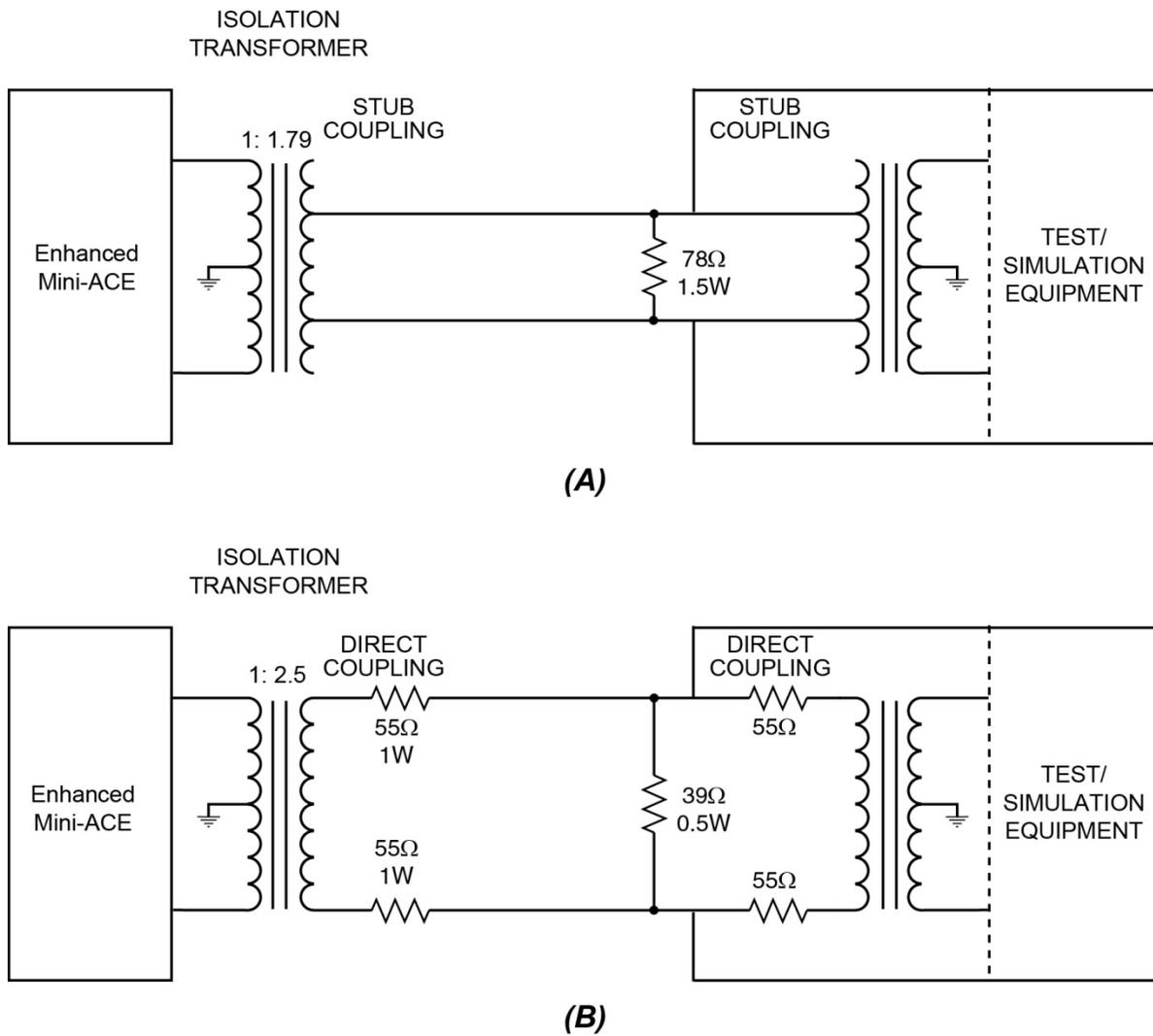
**Figure 14. Simulated Bus Interconnections**
