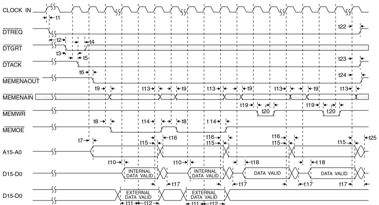
**Figure 48. BC/RT/MT SOM/EOM Burst Read/Write Timing**
