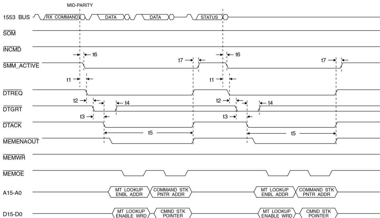
Figure 64. Message MT Command Not Selected Timing
