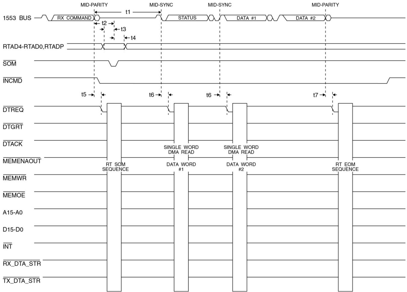
**Figure 57. RT Transmit Message Timing**
