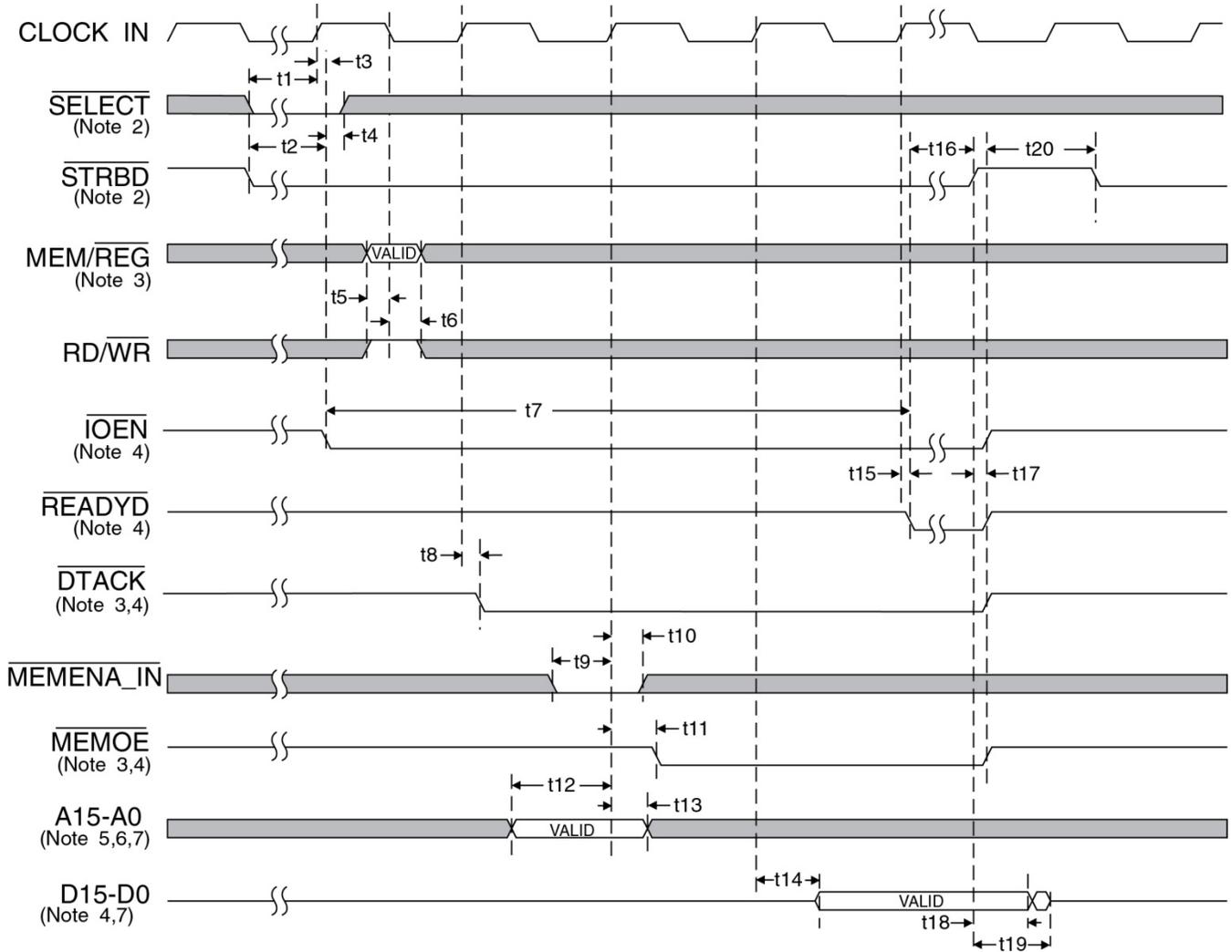
Figure 26. CPU Reading RAM/Registers (Transparent Mode)
