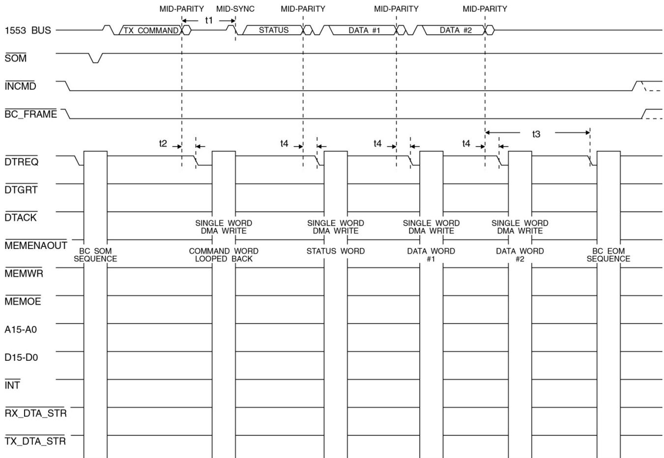
**Figure 50. BC Mode Transmit Message Timing Sequence**
