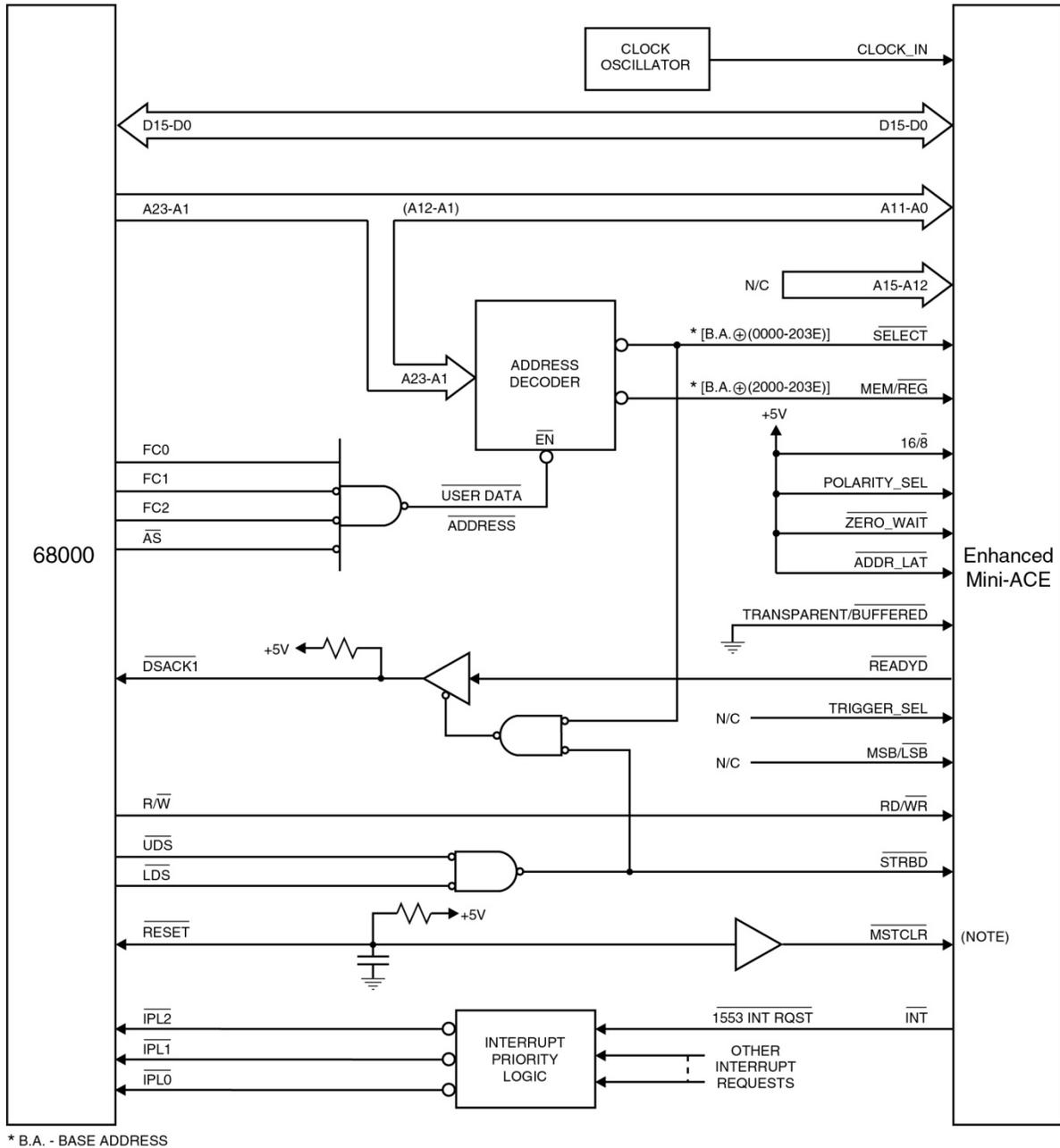
Figure 38. Motorola 68000-to-Enhanced Mini-ACE Interface
