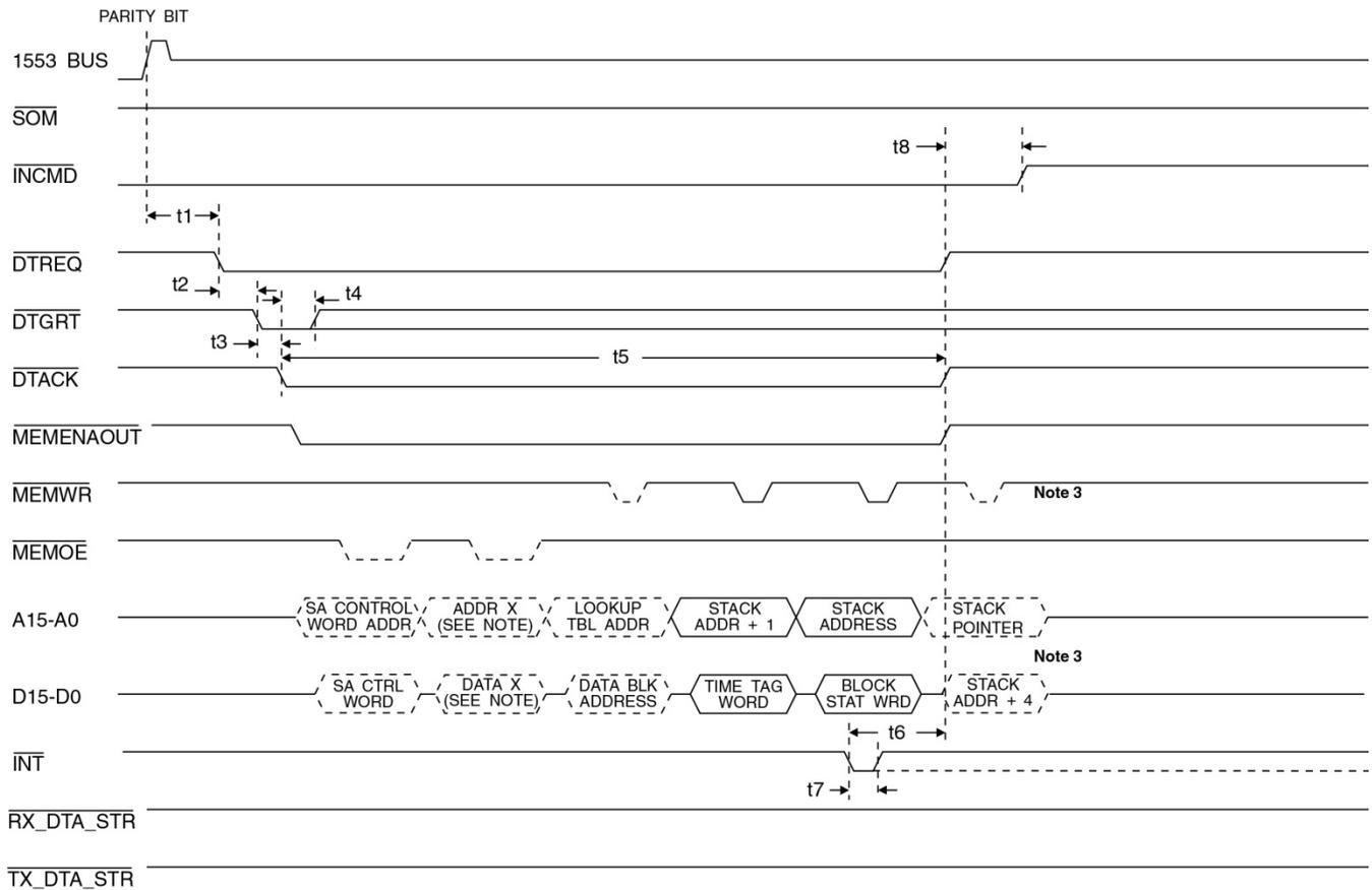
**Figure 60. RT End of Message (EOM) Timing**
