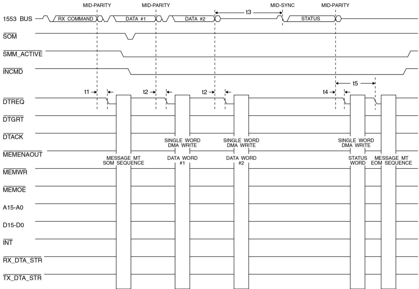
**Figure 61. Message MT Receive Message Timing**
