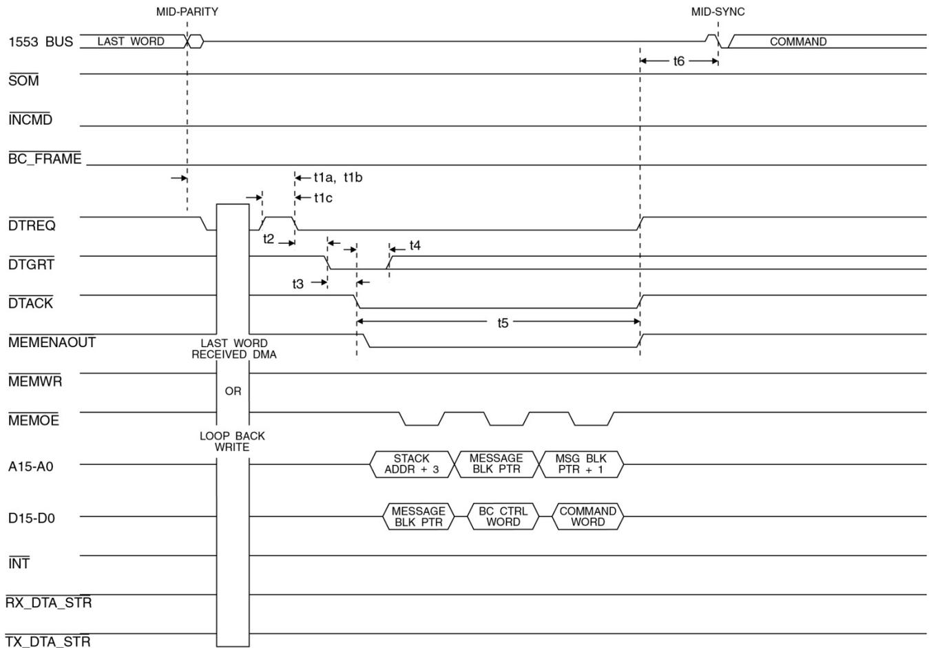
**Figure 55. BC Retry Timing**
