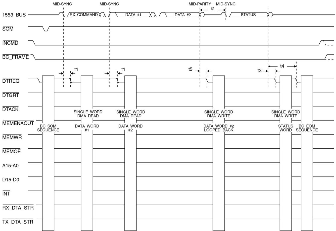
**Figure 49. BC Mode Receive Message Timing Sequence**
