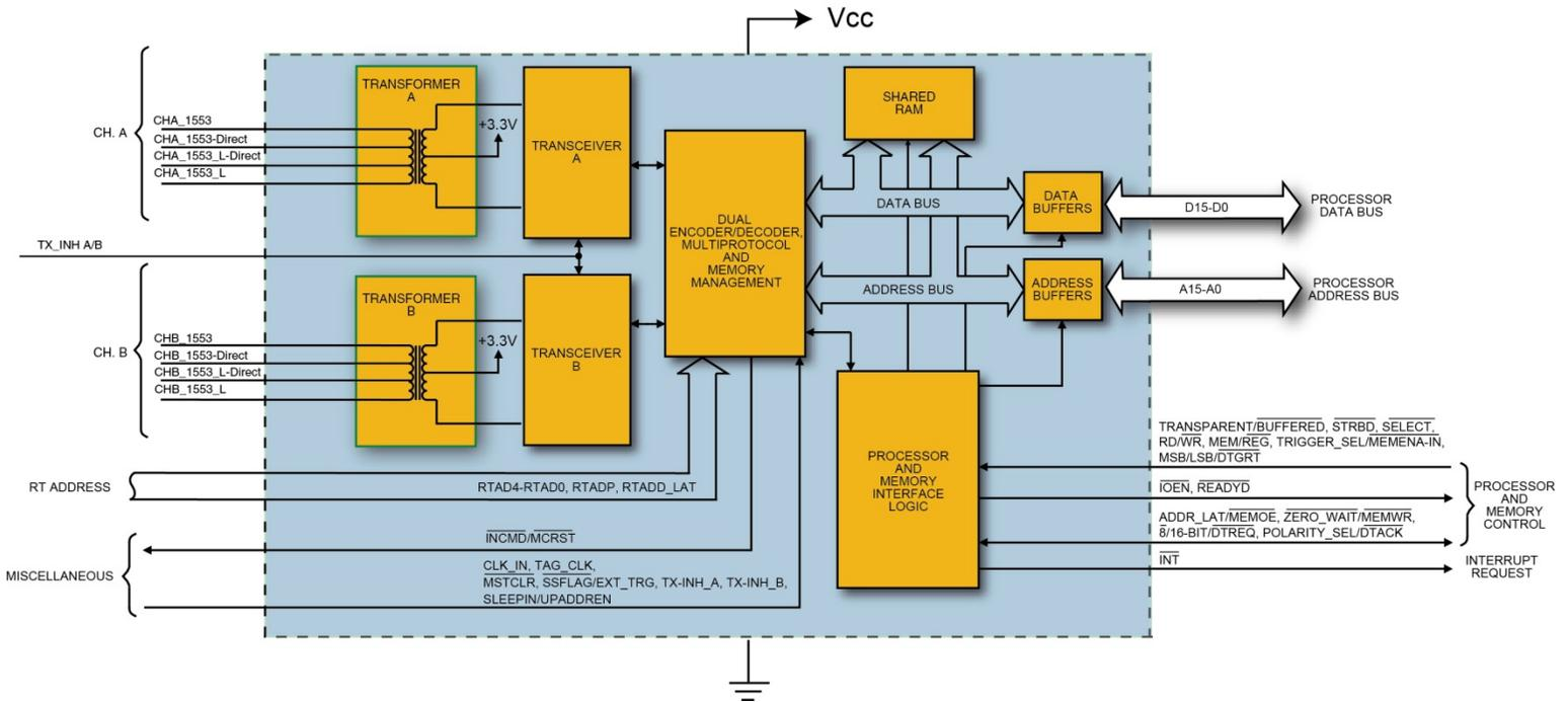
Figure 3. Total-ACE Block Diagram
