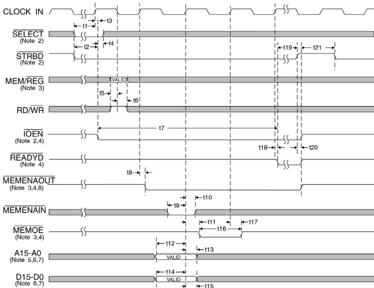
**Figure 27. CPU Writing RAM/Registers (Transparent Mode)**
