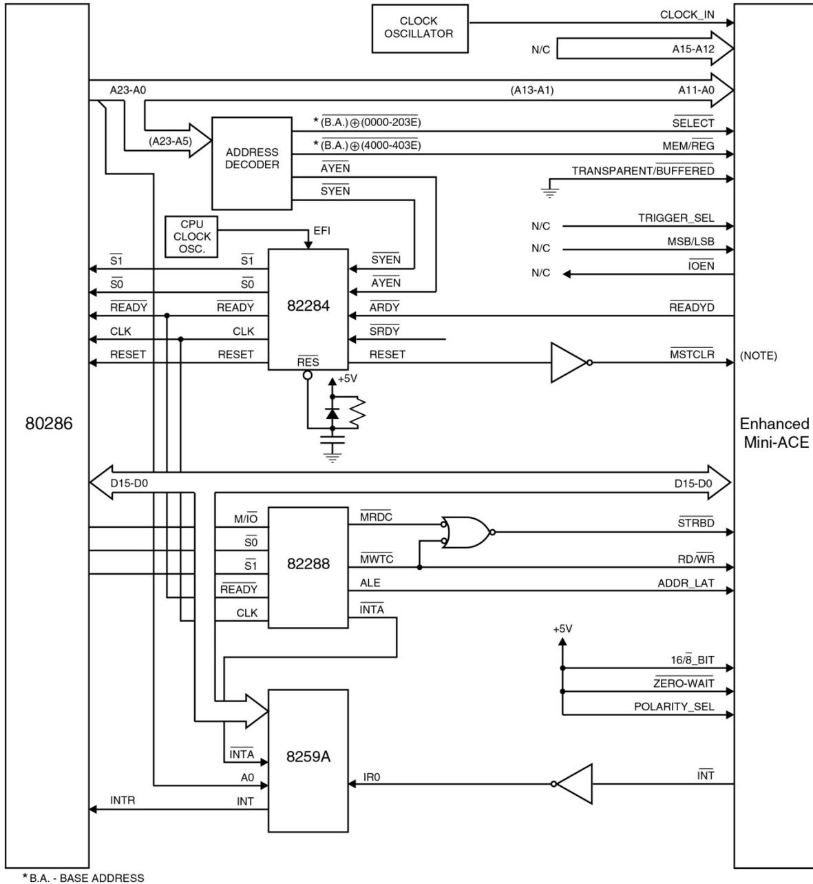
Figure 40. INTEL 80286-to-Enhanced Mini-ACE Interface
