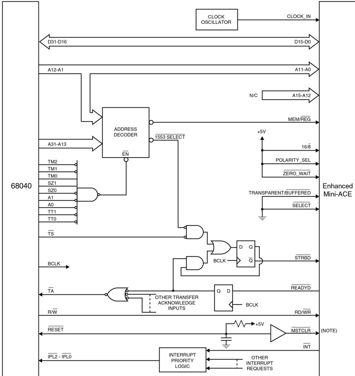
NOTE: The rise time for MSTCLR must be less than 10  $\mu$ s in order to ensure correct initialization of the Enhanced Mini-ACE's Transceivers.
