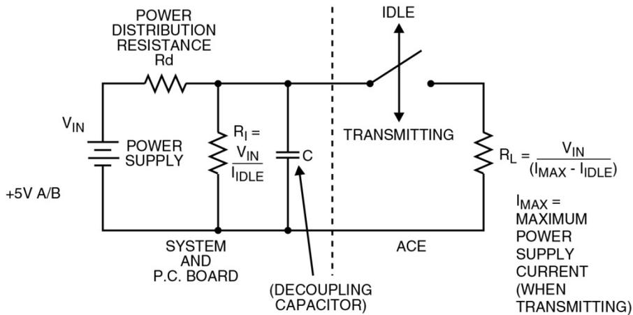
Figure 13. Simplified Equivalent Circuit of Enhanced Mini-ACE Terminal
