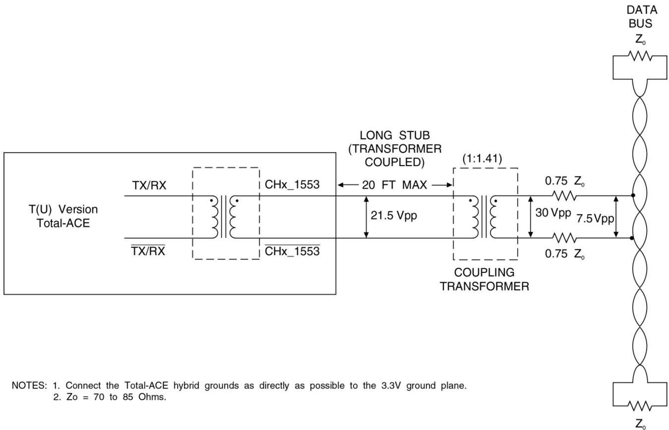
**Figure 7. Total-ACE Series Interface to 1553 Bus
