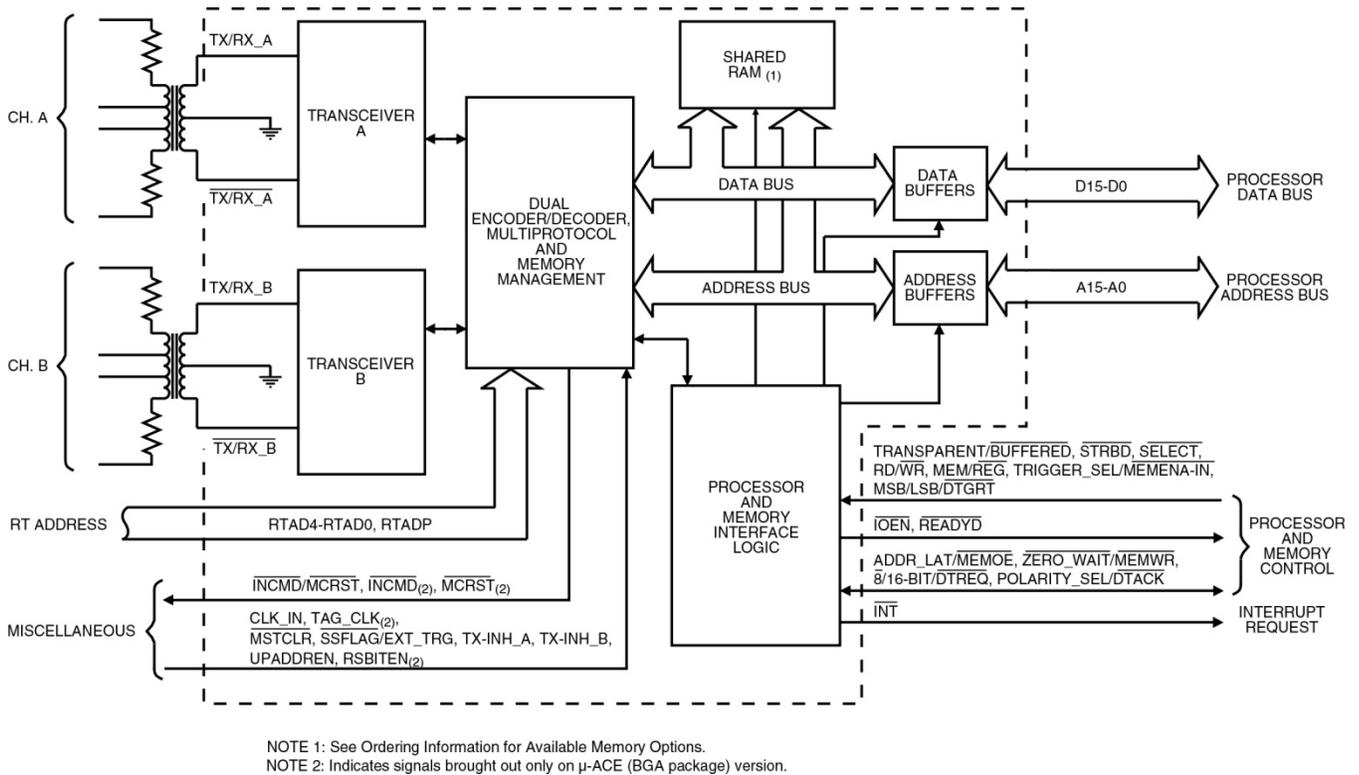
Figure 1. Enhanced Mini-ACE/Micro-ACE Series Block Diagram
