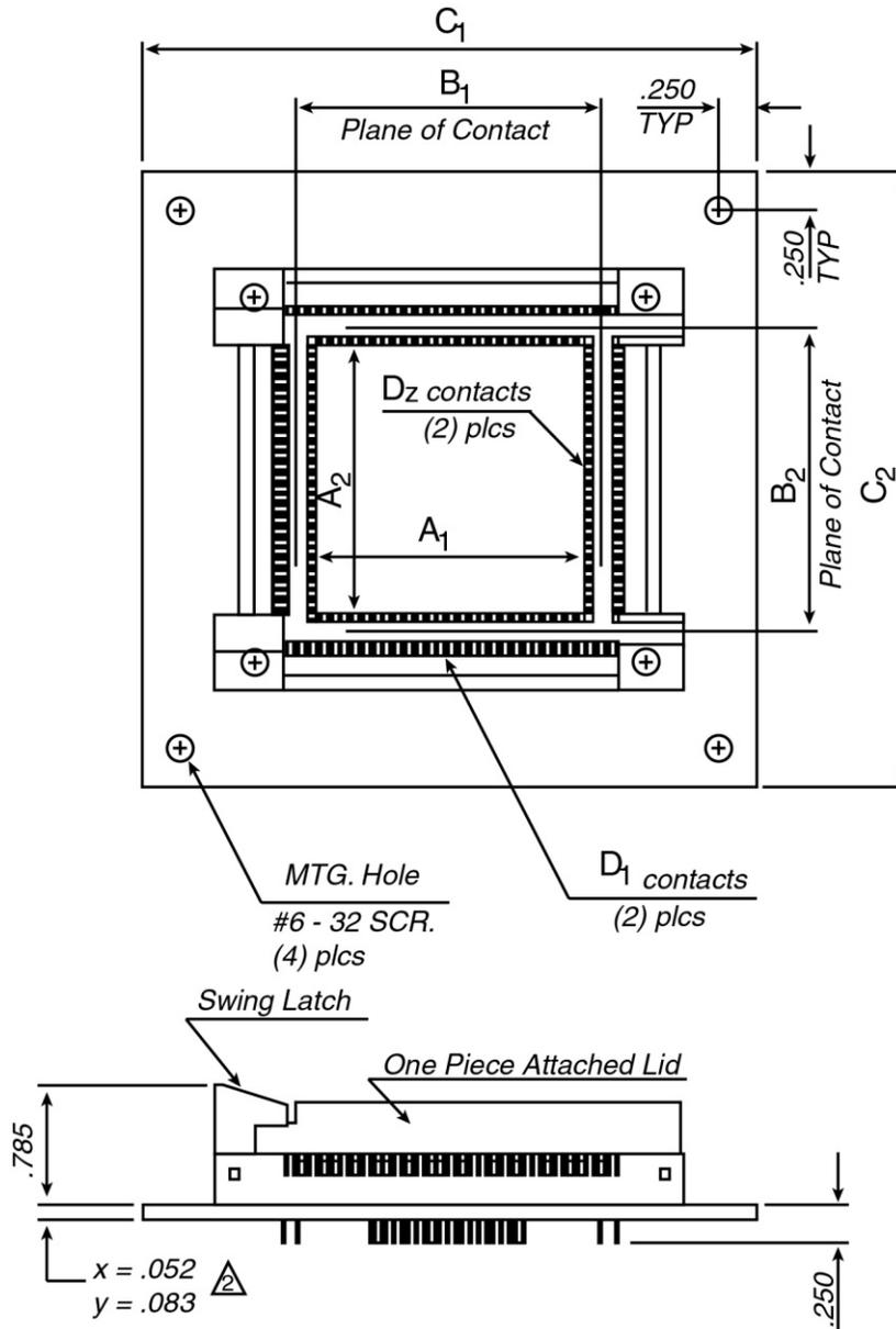
**Azimuth 72-Lead CQFP Socket Test, Flat Pack, 6224-53-21X**
