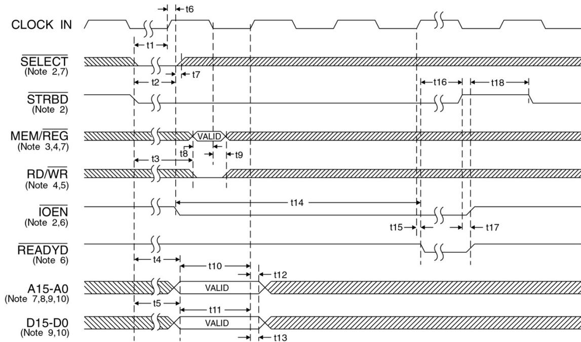
**Figure 23. CPU Writing RAM/Registers (16-Bit, Buffered, Nonzero Wait)**
