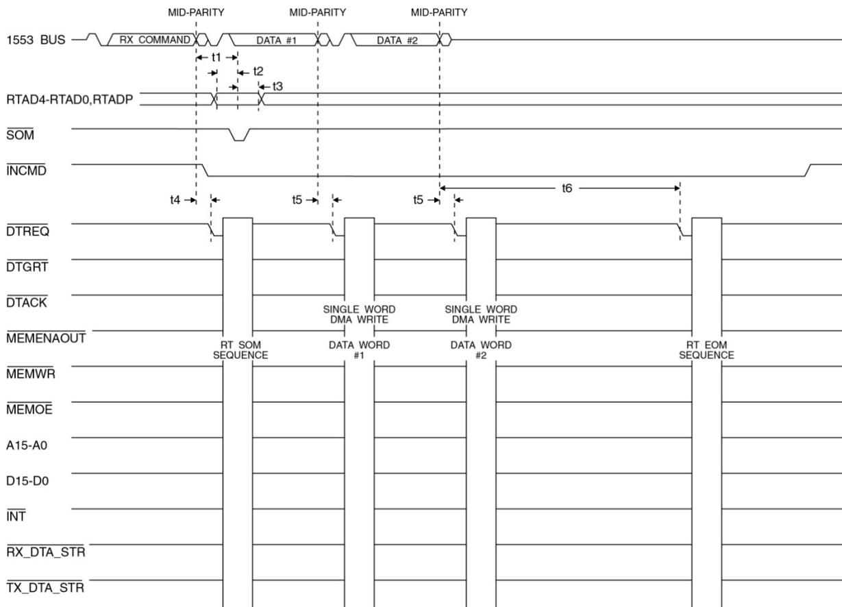
Figure 63. Message MT Broadcast Receive Message Timing
