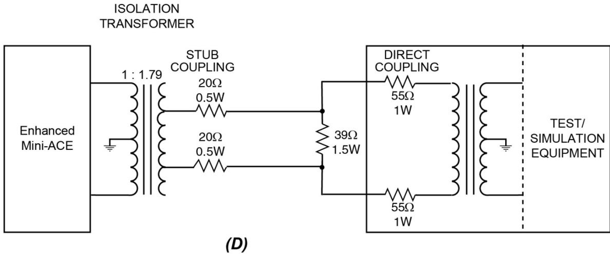
**Figure 14. Simulated Bus Interconnections**
