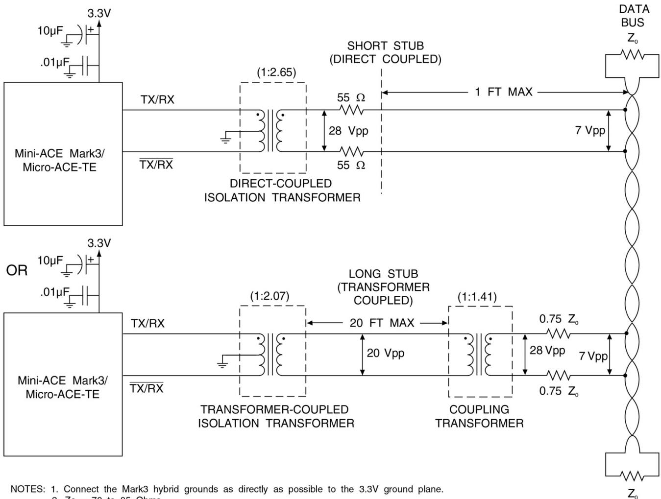
NOTES: 1. Connect the Mark3 hybrid grounds as directly as possible to the 3.3V ground plane.
