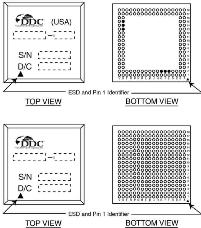
Figure 8. Ball Locations for Micro-ACE-TE and Micro-ACE (BGA Packages)
