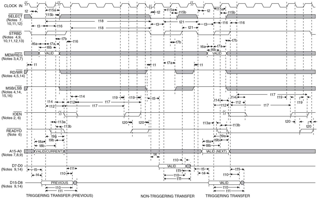
**Figure 30. CPU Reading RAM/Registers (8-Bit, Zero Wait)**
