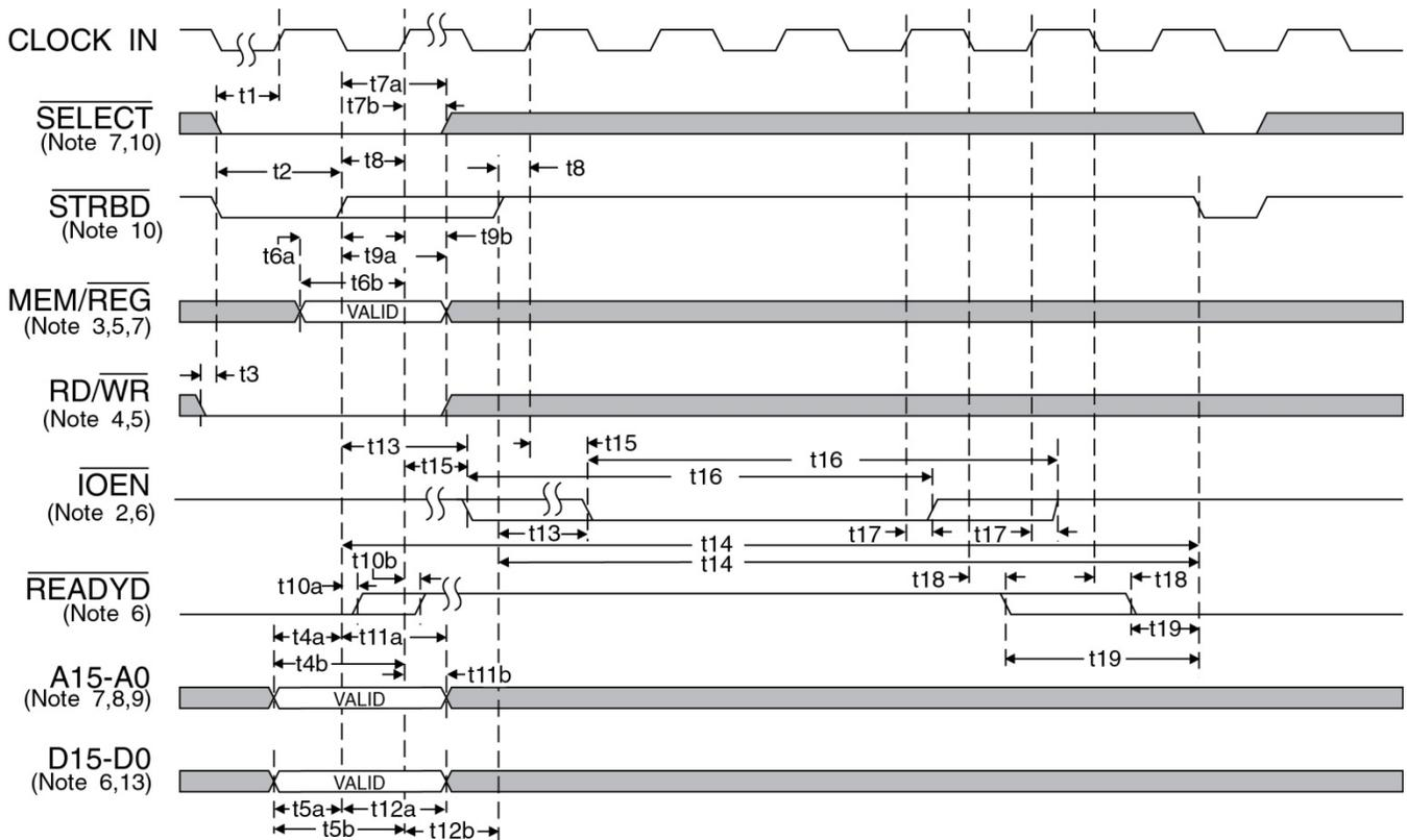
**Figure 25. CPU Writing RAM/Registers (16-Bit, Buffered, Zero Wait)**
