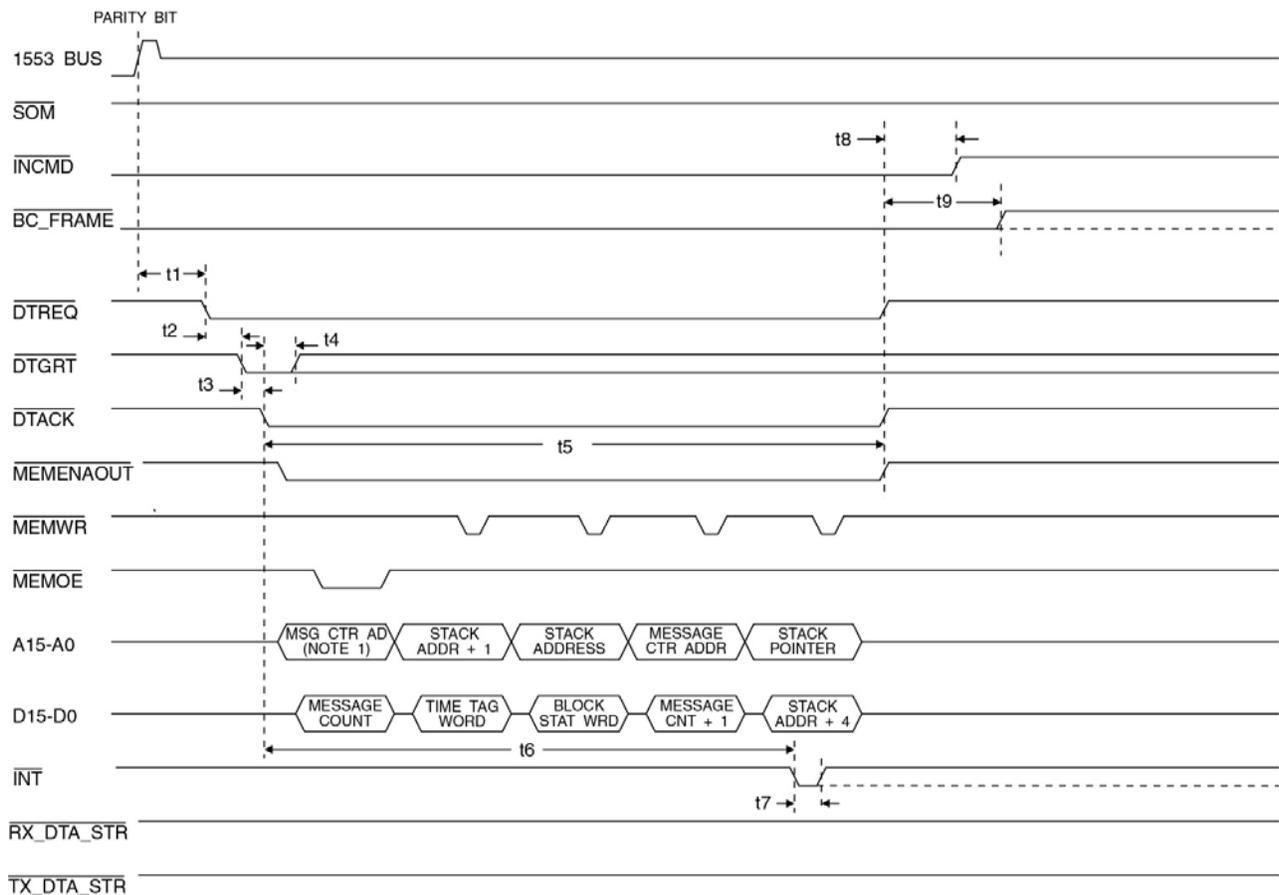
Figure 54. BC End of Message (EOM) Sequence Timing
