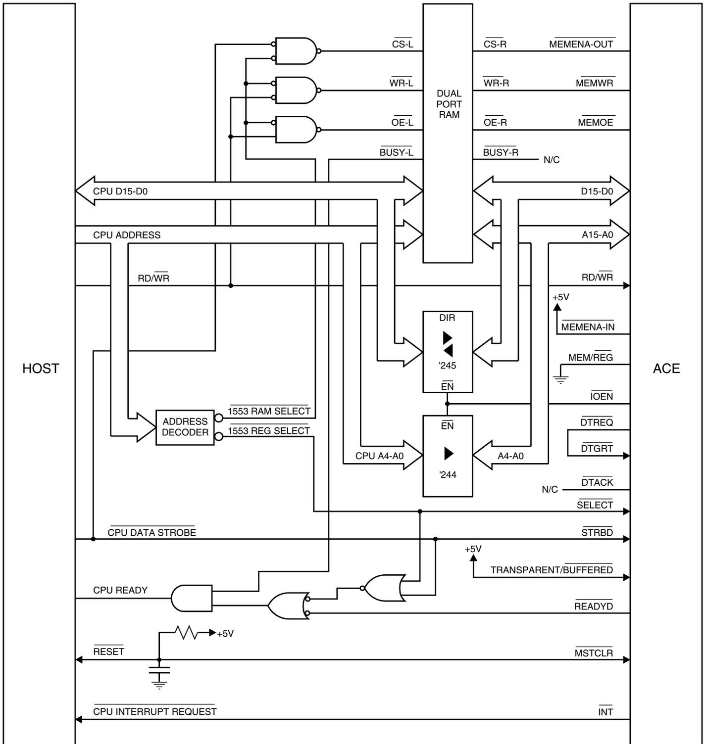
FIGURE 11. 16-BIT TRANSPARENT MODE USING DUAL PORT RAM
