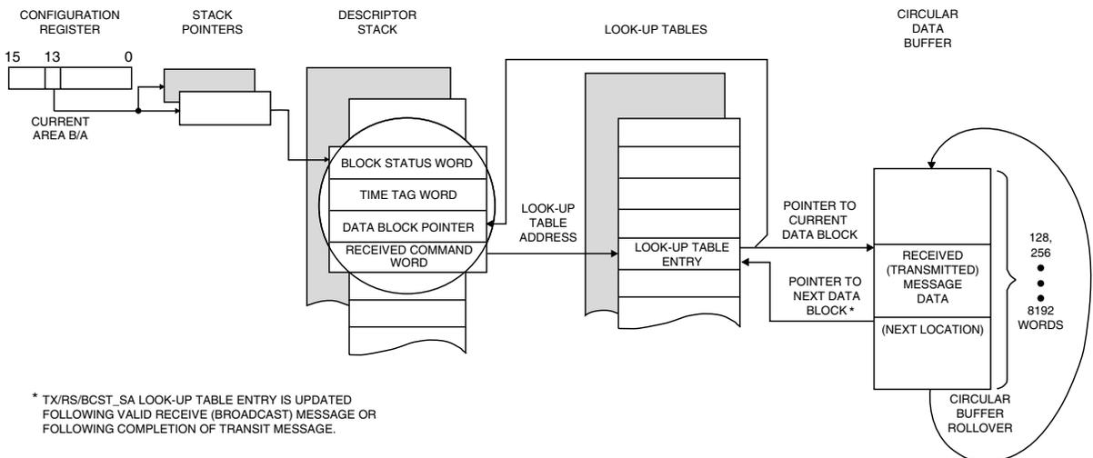
**FIGURE 6. RT MEMORY MANAGEMENT: CIRCULAR BUFFER MODE**
