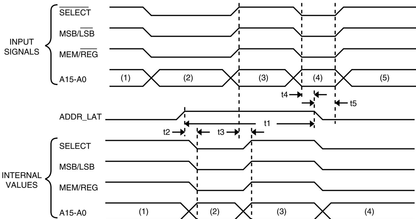
**FIGURE 17. ADDRESS LATCH TIMING**
