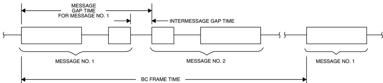
FIGURE 2. BC MESSAGE GAP AND FRAME TIMING
