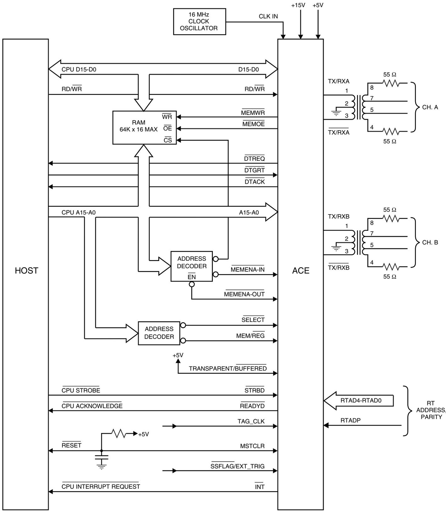
FIGURE 12. 16-BIT DIRECT MEMORY ACCESS (DMA) MODE
