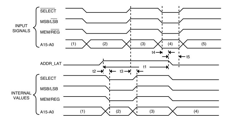
FIGURE 17. ADDRESS LATCH TIMING
