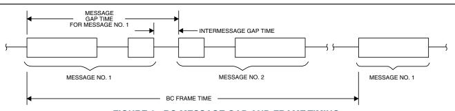
FIGURE 2. BC MESSAGE GAP AND FRAME TIMING
