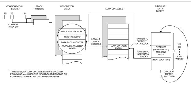
FIGURE 6. RT MEMORY MANAGEMENT: CIRCULAR BUFFER MODE
