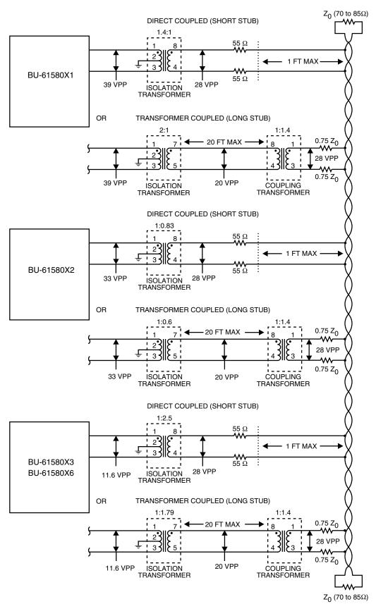
Note: The BU-65170XX, BU-61581XX, BU-61581XX, BU-61585XX and BU-61586XX models are interfaced the same as the corresponding BU-61580XX model is shown (i.e. The BU-65170X1 is interfaced the same as the BU-61580X1).
