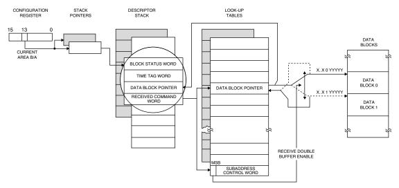
FIGURE 7. RT MEMORY MANAGEMENT: SUBADDRESS DOUBLE BUFFERING MODE
