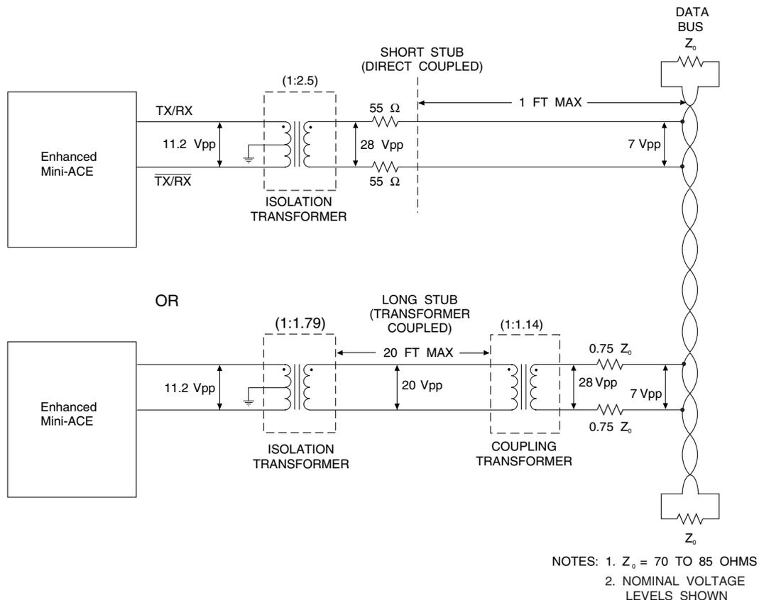
**FIGURE 18. PCI ENHANCED MINI-ACE INTERFACE TO MIL-STD-1553 BUS**
