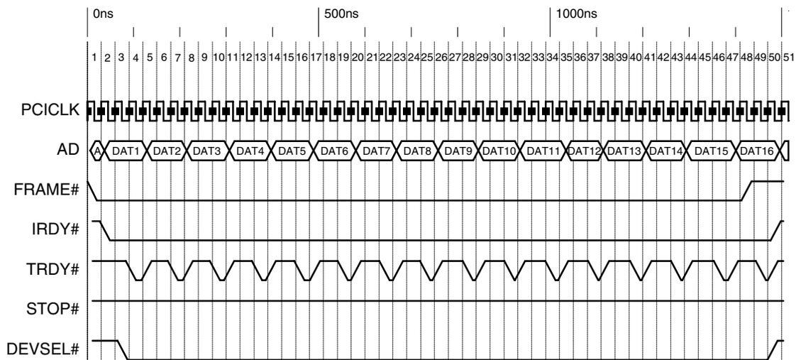
PCI write burst to ACE memory with FIFO empty
