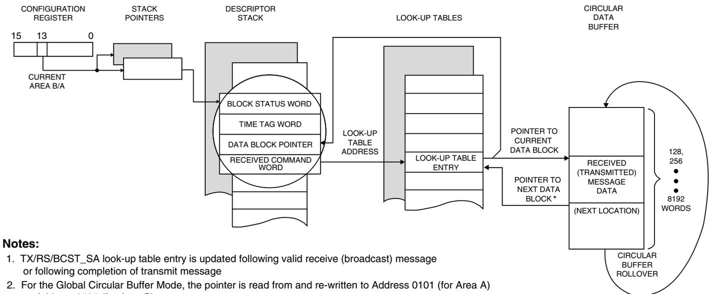
FIGURE 7. RT CIRCULAR BUFFERED MODE
