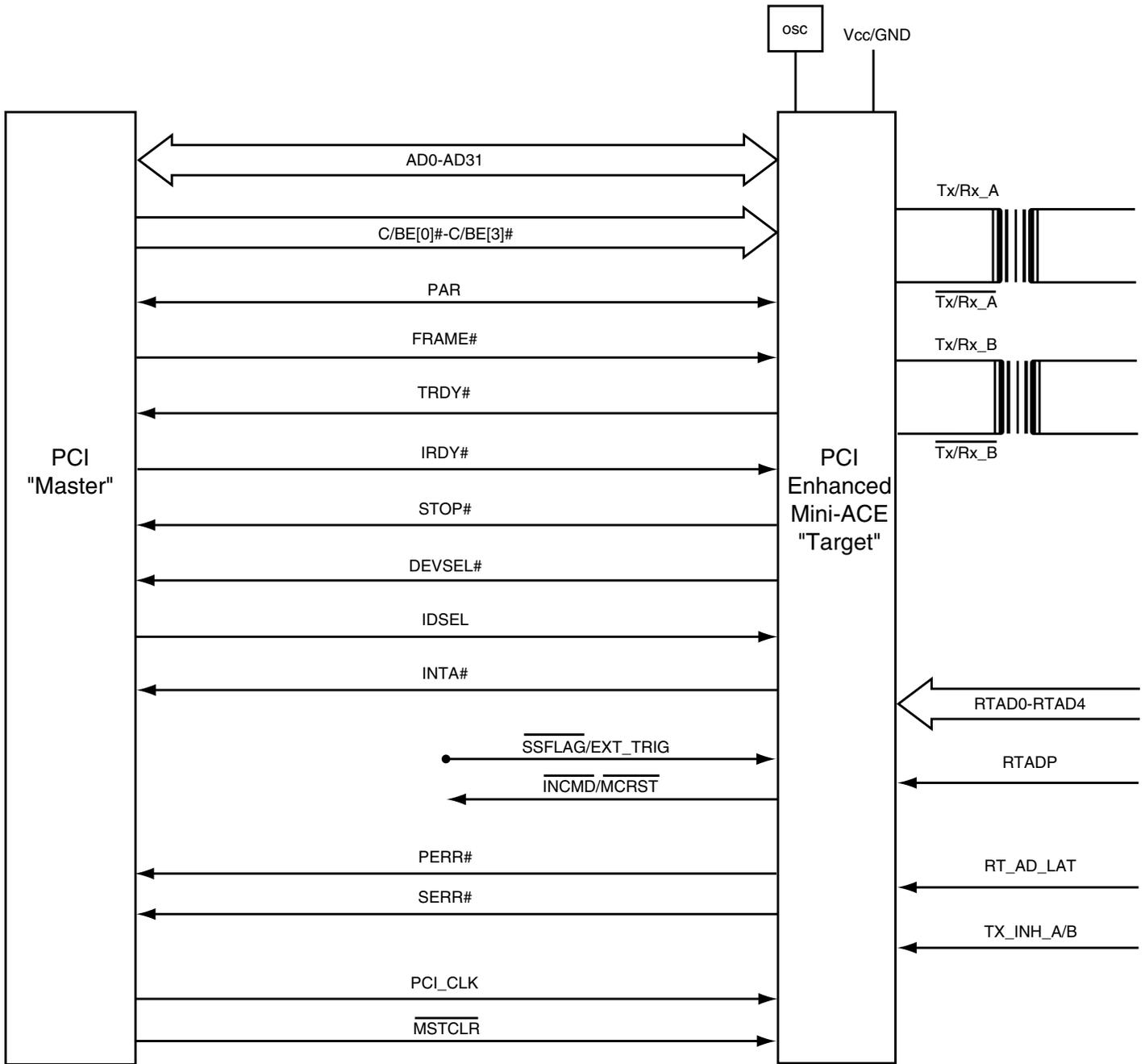
**FIGURE 11. PCI INITIATOR TO PCI ENHANCED MINI-ACE TARGET INTERFACE**
