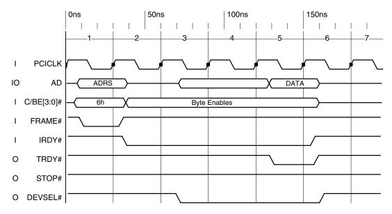
PCI memory read from PCI-ACE interface register space (BAR1 800-81Ch)
