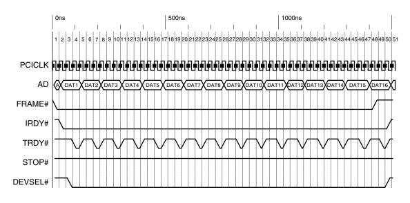
PCI write burst to ACE memory with FIFO empty
