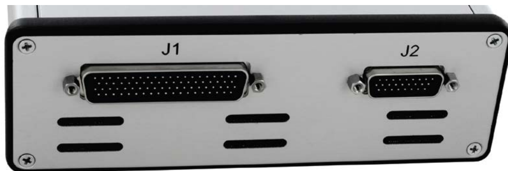
Figure 12. BU-67119WX J1 and J2 I/O Connectors
