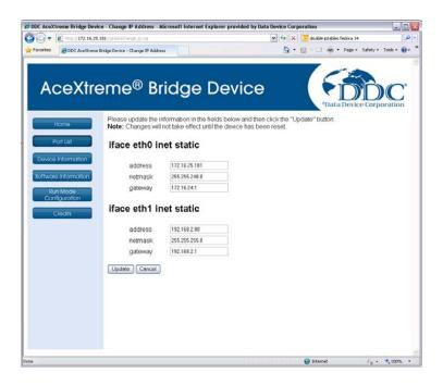
Figure 4. Changing IP Address through Web Server
