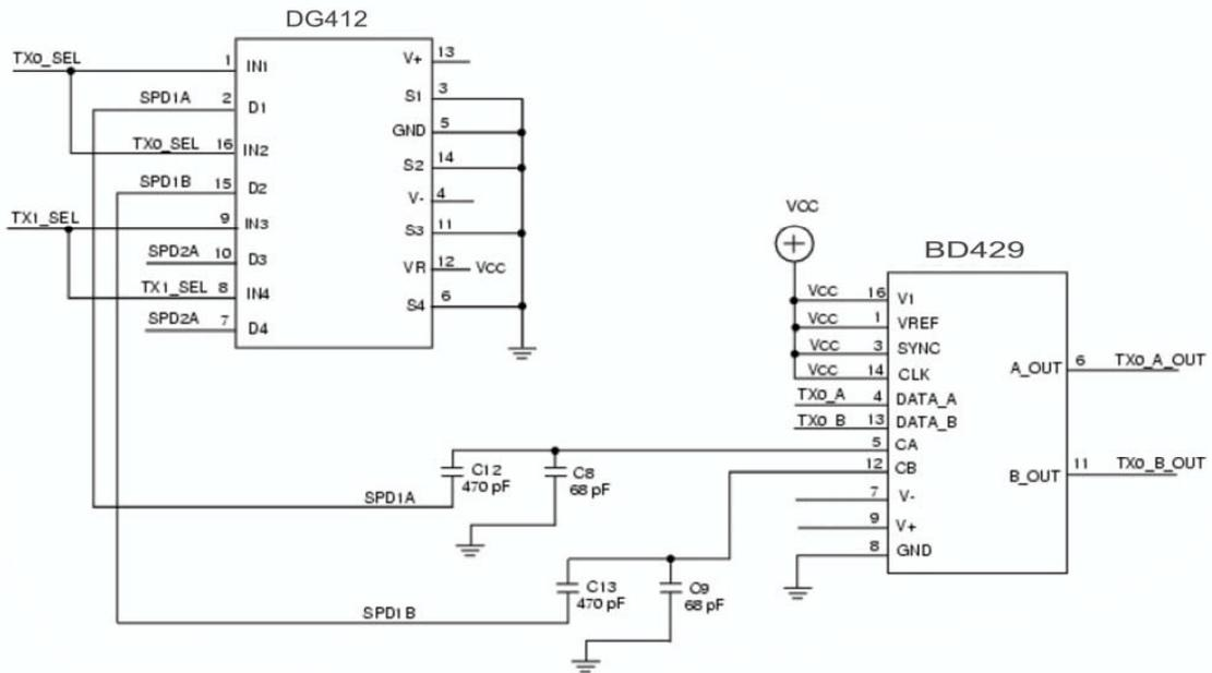
**Figure 8: Typical Circuitry – Switching Capacitors for High-Speed/Low-Speed Operation**
