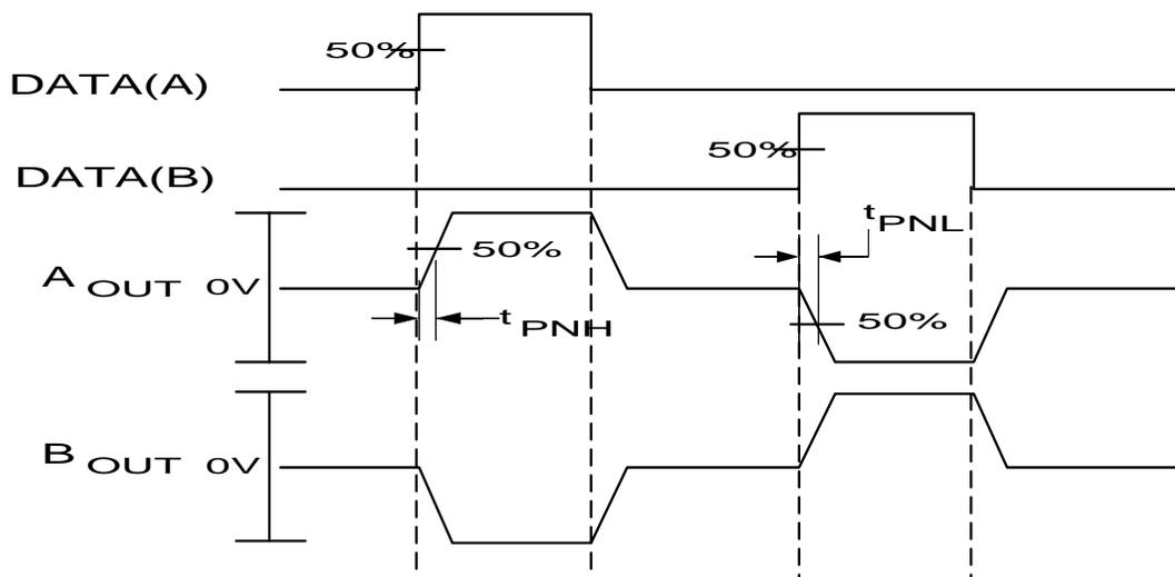
Figure 6: Propagation Delay
