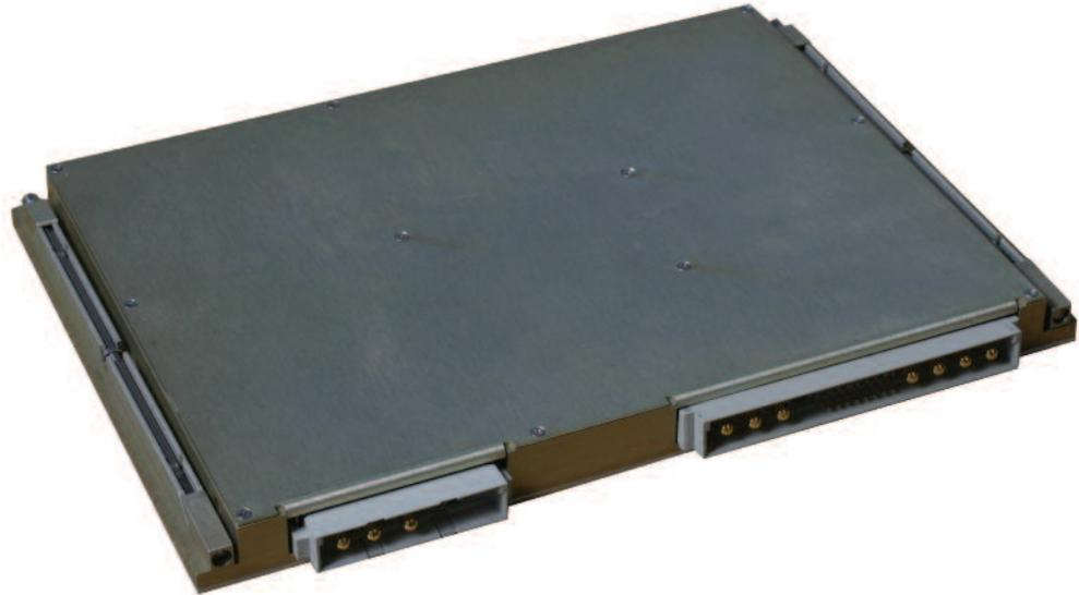
**Input Voltage 85 – 135 V AC, Single Phase 320 – 480Hz**
