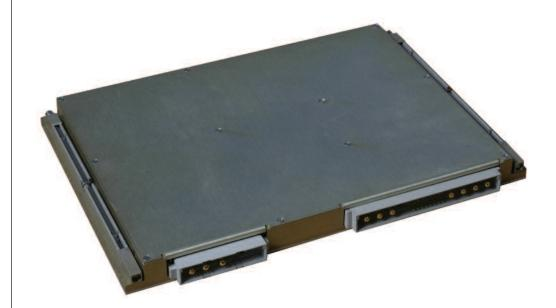
Input Voltage 85-135 V AC, Single Phase 320-480Hz 17.8mm (0.7") profile VME compatible AC FAIL and SYSRESET lines 250W, 5V/30A, 3.3V/10A,  $\pm 12$ V/2.5A, 5V STANDBY/0.1A True current sharing 4ms hold-up capability EMI to MIL-STD-461D -55°C to +85°C operation
