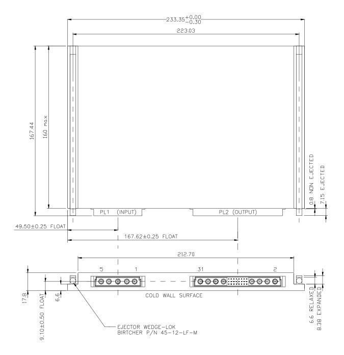
ALL DIMENSIONS IN MILLIMETRES TOLERANCES (UNLESS SHOWN OTHERWISE) DIMENSIONS TO 1 DEC. PLACE ±0.15 DIMENSIONS TO 2 DEC. PLACE ±0.07 OTHER DIMENSIONS ±0.5
