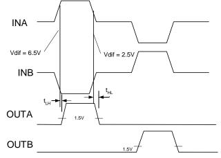
Figure 3 ARINC 429 Input to Logic Output Switching Waveform
