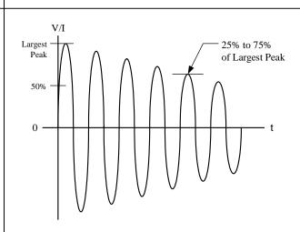
Figure 6 DO160 Lightning Induced Transient Voltage Waveform #3 Pin Injection Voc = 600 V, Isc = 24 A. Freq = 1 MHZ ±20%
