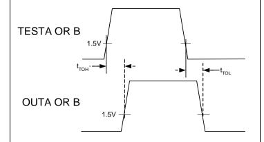
Figure 4 TEST Input to Logic Output Switching Waveform
