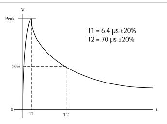
Figure 5 DO160 Lightning Induced Transient Voltage Waveform #4 Pin Injection Voc = 300 V, Isc = 60 A.
