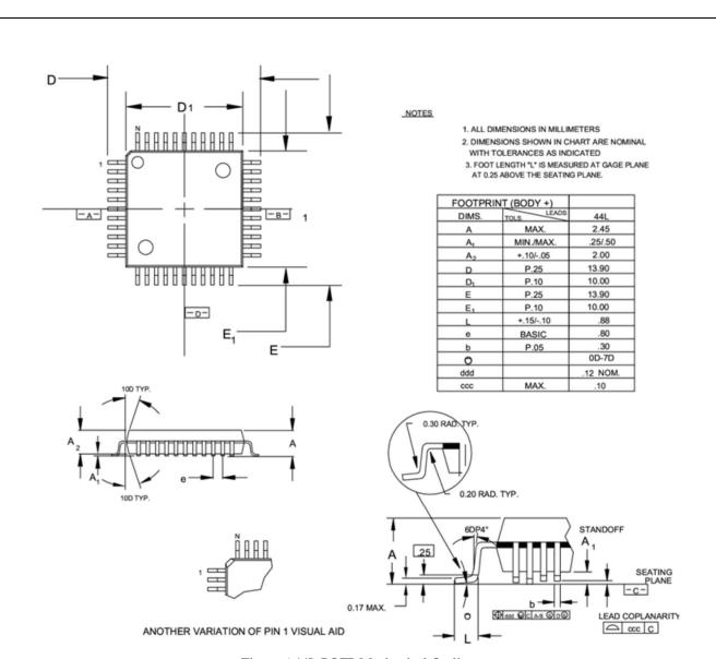
Figure 6 44L PQFP Mechanical Outline
