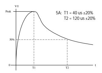
Figure 5 DO160 Lightning Induced Transient Voltage Waveform #5A Pin Injection. Voc = 300 V, lsc = 300 A
