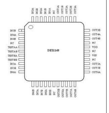
Figure 1 DEI1148 Pinout
