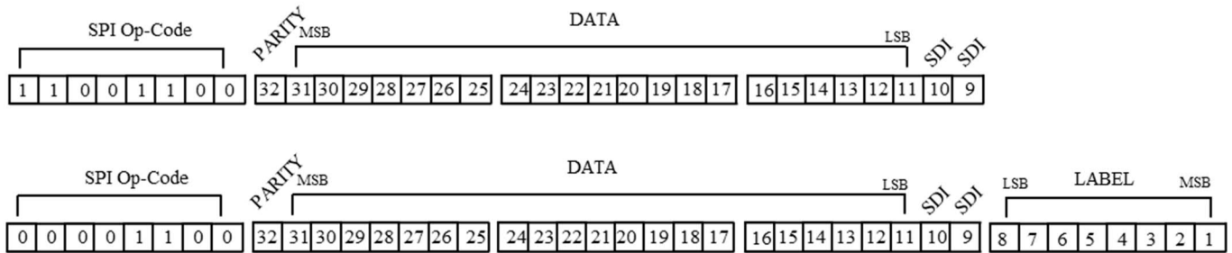
Write Transmit FIFO (Op-Code 0x0C) with TFLIP bit = “0”
