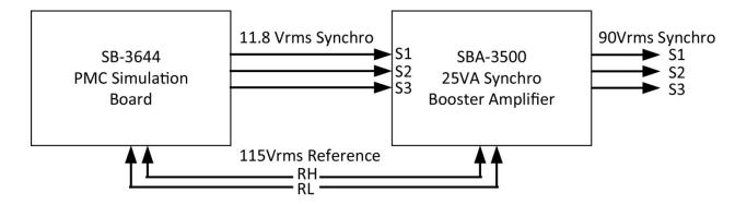
Figure 4. SB-3644 and SBA-3500 Block Diagram
