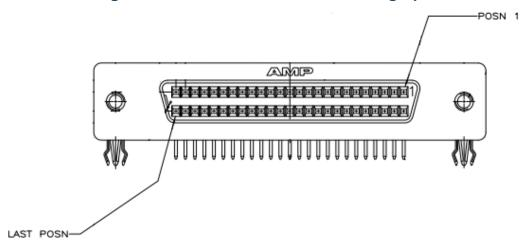
Figure 7. 68-Pin I/O Connector Pin Locations (Viewed from front panel of card, 1 to 34 top row, 35 to 68 bottom row)
