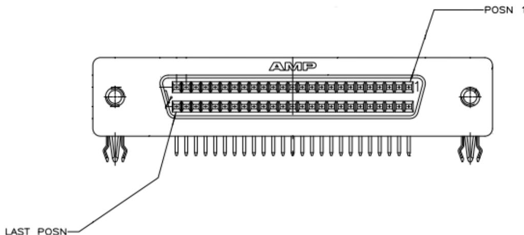
Figure 7. 68-Pin I/O Connector Pin Locations
