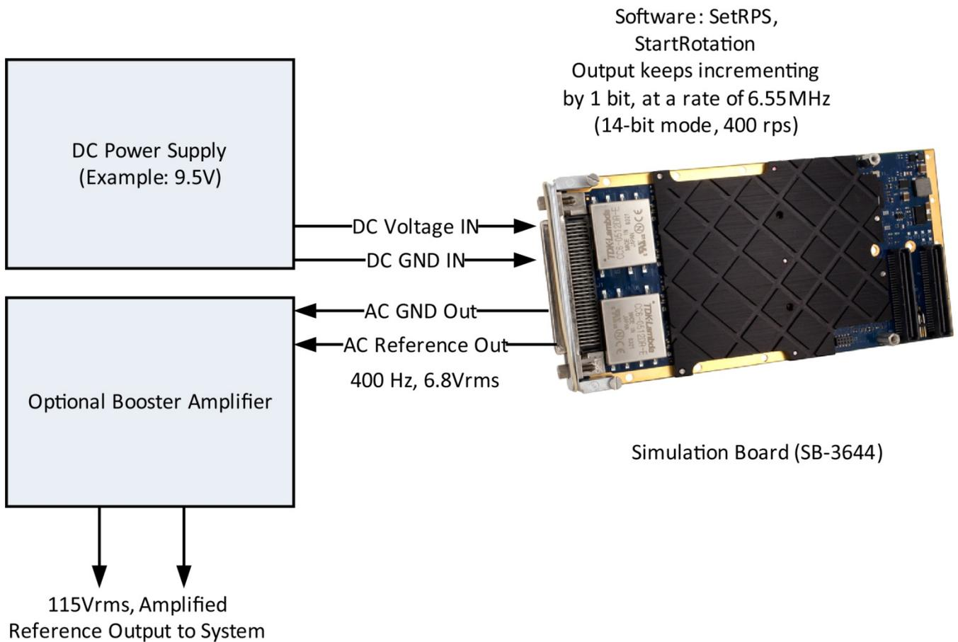
**Figure 5. Simulation Board used as Sine Reference Oscillator Block Diagram**
