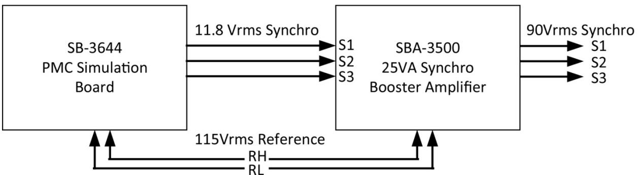
Figure 4. SB-3644 and SBA-3500 Block Diagram
