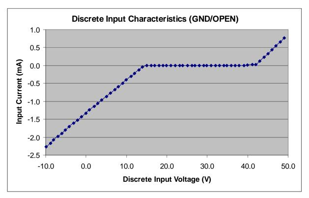
Figure 10 Input IV Characteristics (VDD=15 V)
