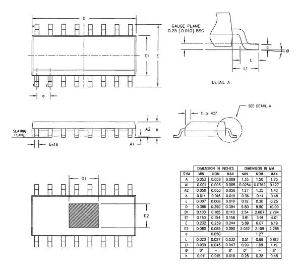
Figure 12 16 Lead Narrow Body EP SOIC Outline
