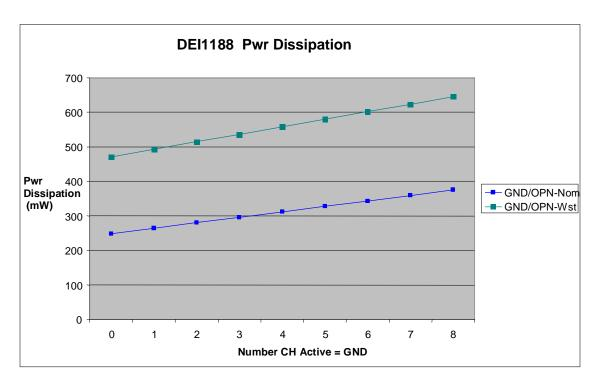
Figure 11 Power Dissipation for Various Conditions
